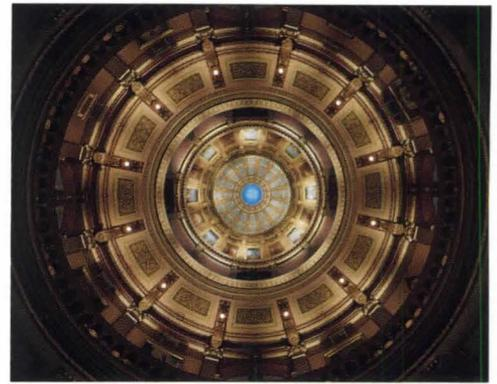
*The lower rotunda (upper left) is illuminated by uplighting through the glass floor, new PAR30 uplights recessed into the floor, existing architectural brackets, and spill from the flag cases and portrait lighting. The upper rotunda (above) is washed by concealed PAR30s and metal-halide spots. The restored architectural wall brackets and floor uplighting wash the walls on the second floor of the rotunda. Existing harps (lower left) light a stairway.*
