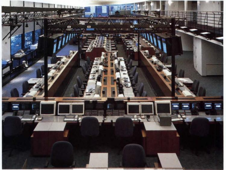
*fixtures mounted on the window wall. Does daylight present a screen-glare problem? The room faces north and the gray solar glazing is 1/2-in.-thick. If all else fails, there are shades. A fiber-optic strip behind the edge of the ceiling cove makes it appear to float.*
