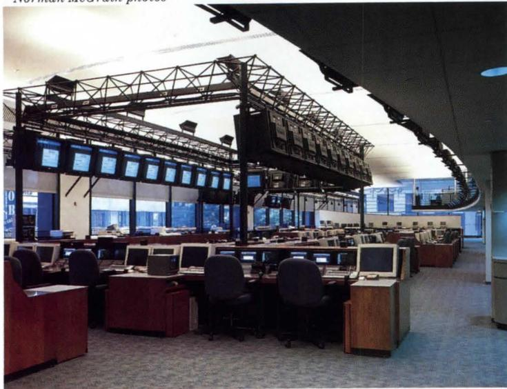
*The halogen uplights are a type usually used outdoors. Project architect John Kinnear designed baffling for the tops of fixtures to conceal the intensely bright lamps from the view of persons standing on the mezzanine. A slanted, smaller-scale baffle was used to shield*
