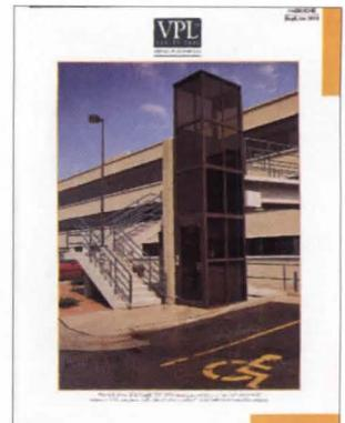
The VPL™ Series 2000 Vertical Platform Lifts from the Cheney division of Access Industries, Inc. provide stairway access indoors and out for people who use wheelchairs. Lifting heights from 1" to 144" for loads up to 750 lbs. are available for both commercial and residential applications. Easy to install and operate, the units are space and cost efficient solutions to ADA access compliance. Attendant operation, toe-guard enclosure and restricted access hoistway enclosure options are available.
