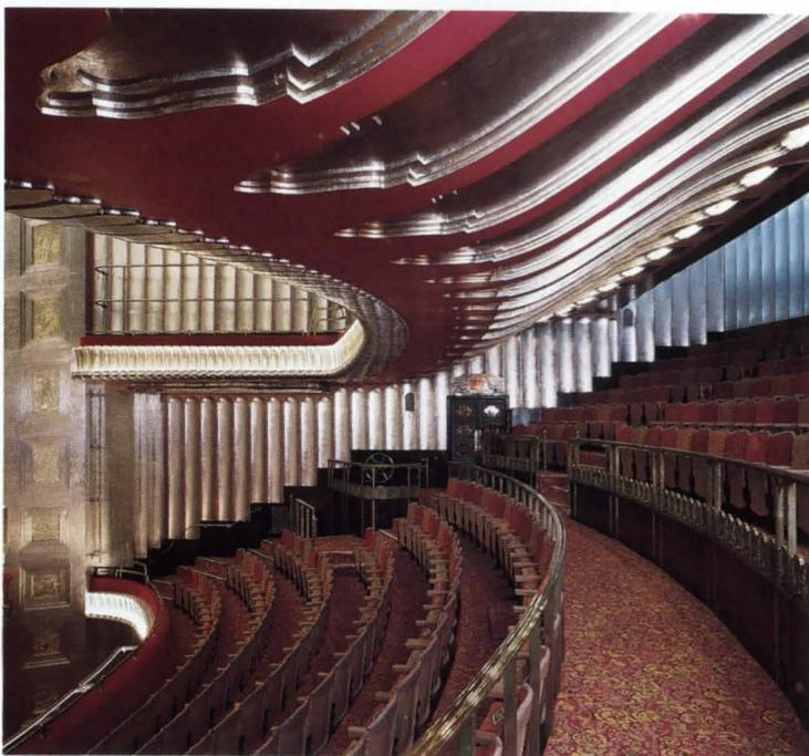
*Dramatic lighting makes full play of the Savoy's aluminum-leaf decoration. Long-life tungsten lamps are used in the ornate ceiling coffers over the stage and along the balcony fronts, while cold cathode gently highlights the edges of the balcony ceilings. All the house lighting is controlled by a single dimming system.*
