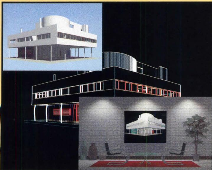
*Rendered view (upper left) can be applied to a surface (lower right) in a ray-traced image from the add-on rendering module.*
