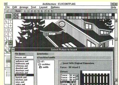
The foreground window shows the process for picking a fence from Abracadata's Architecture module symbols library. The drawing in the background is 2D, rendered in perspective.
