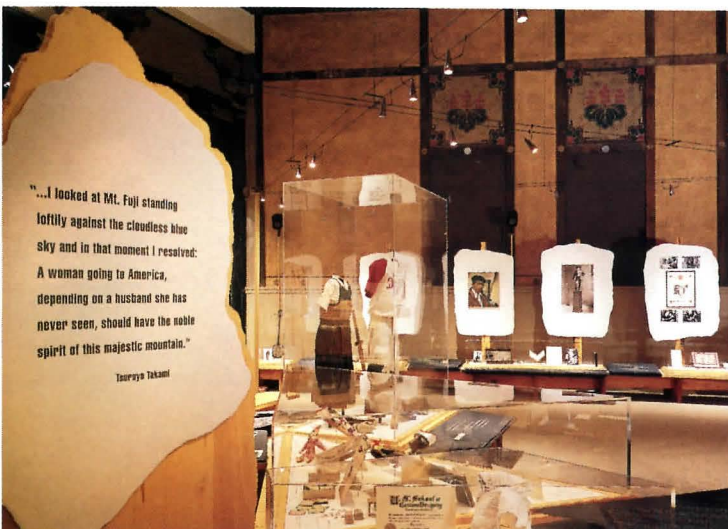
Located in a landmark building where no new ceiling- or wall-mounted fixtures were permitted, the exhibit has been lit with the aid of cables connected to poles standing on a built-up floor. The cone-shaped fixtures use MR16 lamps with UV filters to protect the fragile artifacts.
