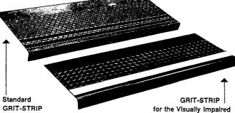
Two 3/4" wide abrasive mineral coated durable grit-strips, which help prevent slipping, are recessed the entire length 1" from front edge.
