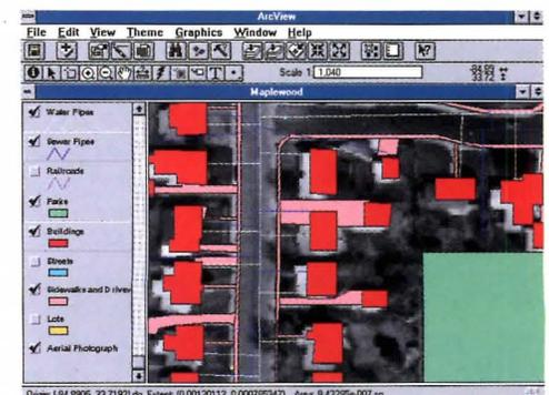
Area of first view, but with sewer pipes and sidewalks added.
