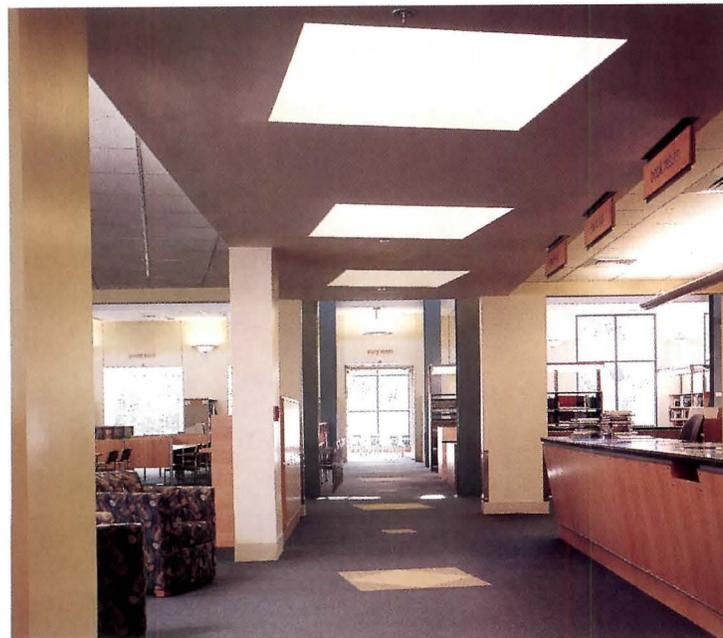
The main reading room or “great hall of books” (left) is a basilica in plan, with stacks in the nave and reading tables in the aisles. Seismic bracing runs along the east and west walls below clerestory windows. The circulation desk (bottom left) offers self-check-out service. The meeting room (opposite) plays host to city council meetings.
