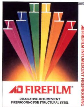
Now Certified for beams and columns for ratings up to 2 hours! A/D Firefilm permits the designer to use the appearance of exposed steel with the steel fully protected from fire. It is applied as a thin-film coating 0.4 to 3 mm (0.02 to 0.12 in.) thick. During a fire A/D Firefilm expands to form a meringue-like layer up to 100 mm thick, which insulates the steel from the fire. The topcoat is available in a wide choice of colours.
