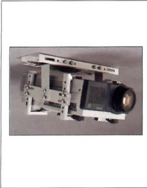
Designed to accommodate LC projectors weighing up to 75 lbs. the new Peerless PJRL30 Projector Mount is adjustable in height (5 5/8" - 9 3/8") and width (10" - 25 3/4"). It features 0° to 10° forward and backward tilt, heavy-gauge steel construction, rubber-lined clamping mechanisms at the four corners, and full 360° rotation when used with the optional extension column. Available in gray or black, the PJRL30, may be mounted directly to the ceiling.
