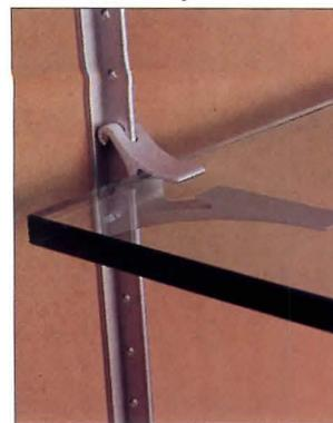
"ellen's brackets", an anodized aluminum shelving system designed by M Ali Tayar, provides an elegant alternative to existing bracket-and-track systems. Cantilevered brackets come in two sizes, for shelves 3/4 or 3/8-in. thick and 10-in. deep. Wall-mounted tracks permit 1/2-in. adjustment of wood, glass or plexiglass shelves.
