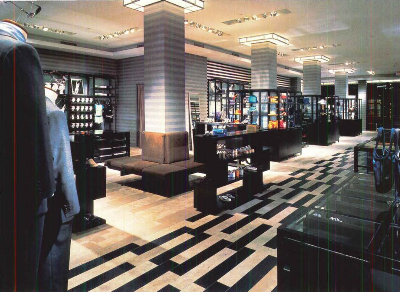
Low-voltage tracks in fluorescent-backlit troughs illuminate clothing in the upper floors (left). Concept drawings (right) show how the front windows and column capitals are lighted.
