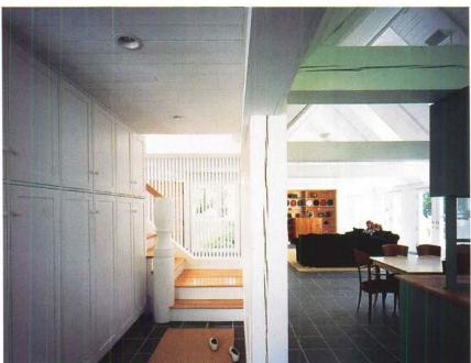
Slate flooring continues the bluestone paving used outside (above). Counters are wood and slate. Vaults in the kitchen and family room are constructed from tie beams recycled from previous use, and the white-painted slatted staircase is in keeping
