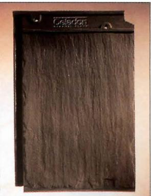
A kiln-fired, interlocking clay roof tile designed to look like thick slate with a breaking strength greater than 300 pounds; impervious to freeze-thaw degradation with less than 1% moisture absorption; color will not fade, flake, or effloresce—offered in slate gray, slate red, montpelier green, plumstone, and brunswick black. Sixty-year limited, transferable warranty. 1-800-699-9988.
