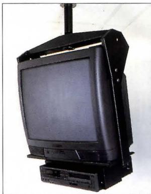
Feature adjustable height, width, tilt & swivel. Mounting plate allows the fine-tuning of gravity in relation to degree of tilt, while top clamps provide stability. Constructed of heavy gauge steel with durable epoxy finish, mounts are avail. in sizes to accom. 13" - 42" screens & 125lb. - 300lb. UL listed & CSA cert. Several OSHPD apprd. VCR attachments & tamper resistant security fasteners opt.
