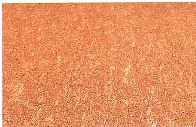
chopped wheat straw and a synthetic polymer resin pressed into long strips. Similar to medium-density fiberboard, Isobord is 15 percent lighter than most wood products and does not use formaldehyde in the manufacturing process. It exceeds ANSI-M3 standards and can be used for countertops, cabinets, and furniture. 503/242-7345. Isobord Enterprises, Elie, Man., Canada. **CIRCLE 228**
