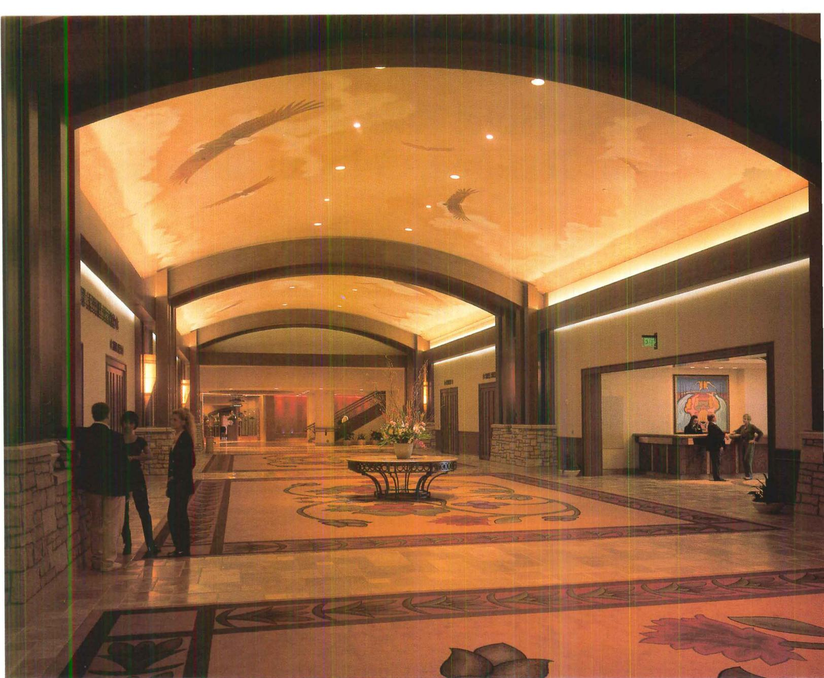
The overall lighting approach “was to light up rather than down,” says Steffy. “We specified uplighting to illuminate covered ceilings, copper chimneys, wood and stone walls, and architectural details including metalwork and moldings.” The intent was to eliminate direct-source glare and impart an upscale ambience; subtle interior lighting
