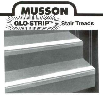
Photoluminescent (Glows in the dark) Glo-Strip<sup>™</sup> is available in any Musson Visually Impaired stair tread. 2" wide white grit-strip is made of non-toxic, non-radioactive zinc-sulfide crystals that absorb, and store light. Luminescence can be seen after lights cease operating; helps lead the way to safety. Recharge by exposing to light. Meets ADA slip resistance and high contrast regulations.
