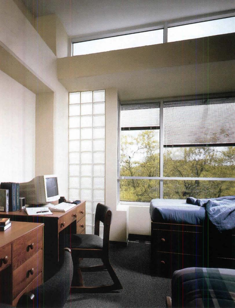
**Window walls with clerestories and glass blocks flood bedrooms and study areas with daylight (left and below). These elements also vary the architectural geometry, an improvement on the “stacked box” housing the structure replaced.**
