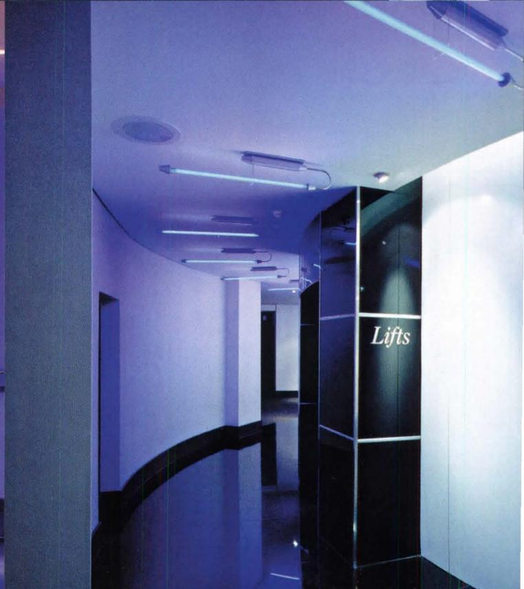
The lighting of the entry of the BT Tower is complex, so several views are shown here. A slot cut into the convex ceiling houses cold-cathode cove lighting used to orient visitors toward the auditorium and conference rooms beyond. Other slots cut
