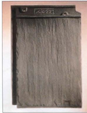
A kiln-fired, interlocking clay roof tile designed to look like thick slate with an average breaking strength of 300 pounds; impervious to freeze-thaw degradation with an average of 1% moisture absorption; color will not fade, flake, or effloresce—offered in slate gray, slate red, montpelier green, plumstone, and brunswick black. Sixty-year limited, transferable warranty. 1-800-CEL-SLATE. [www.certainteed.com](http://www.certainteed.com)
