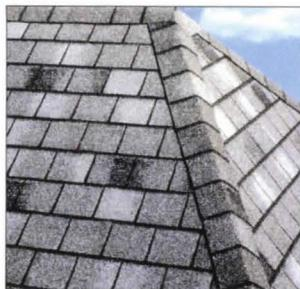
An oversized 18" x 36" fiber-glass asphalt shingle designed to withstand hurricane force winds. Features a dramatic eight-inch exposure; deep one-inch shadow lines; seven colors; and a 40-year limited warranty, including 10-year warranty coverage against winds up to 110 miles per hour. UL certified to meet ASTM D3462 performance standards; Miami-Dade approved; algae resistant.
