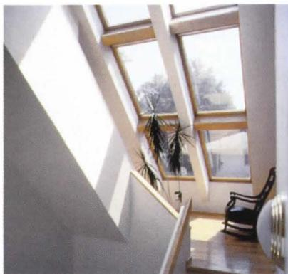
feature a laminated inner pane that provides safety from impact situations, such as hailstorms and high winds. The skylights reflect 99 percent of ultraviolet rays, which can cause carpet and furniture to fade. The glass also has a double layer of Low-E coating to act as a heat barrier. Argon gas, injected between the panes, increases the thermal performance. Velux also offers a selection of pleated shades and
