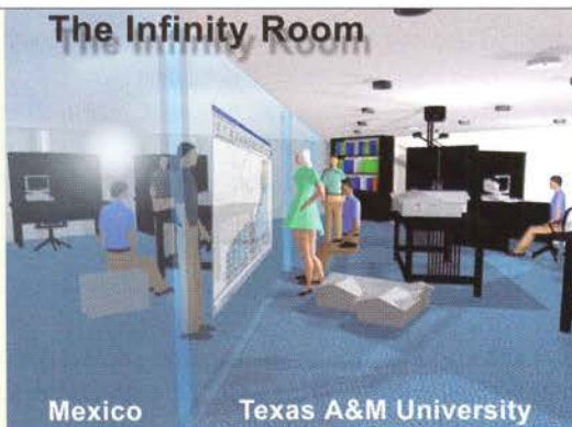
The Infinity Room involves building studios in different locations (plan, right) equipped with floor-to-ceiling rear-projection screens, computers, and video equipment to create life-size images.
