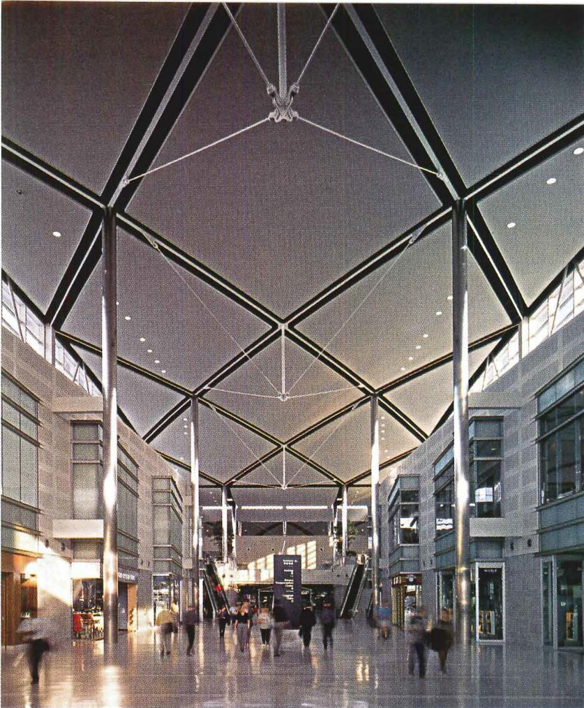
With ceilings rising as high as 70 feet and a diagonal king-post truss system that allows structural spans of up to 87 feet, the terminal's interiors (this page) feel spacious and offer long views that help passengers orient themselves. An overhead tram runs in the terminal itself (opposite), rather than between terminals, making connections between gates faster.
