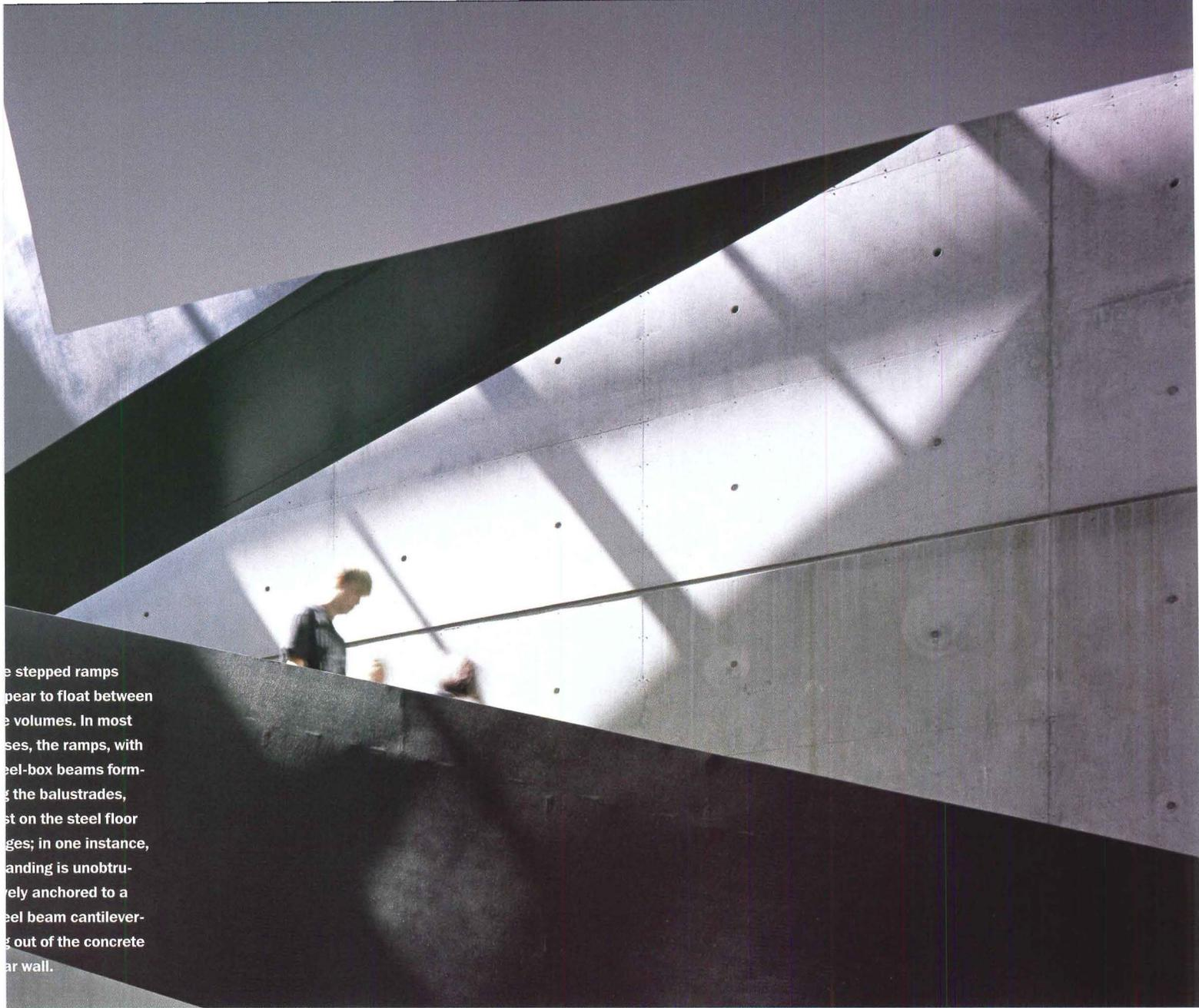
the stepped ramps appear to float between the volumes. In most cases, the ramps, with steel-box beams forming the balustrades, rest on the steel floor joists; in one instance, the railing is unobtrusively anchored to a steel beam cantilevering out of the concrete stair wall.
