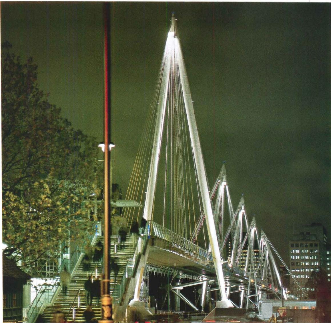
Pylons are backlit by narrow-angle spotlights, 70-watt fixtures focused upward and 30-watt fixtures grazing downward (left). Spotlights with spread lenses and 150-watt lamps illuminate the cable stays (below).
