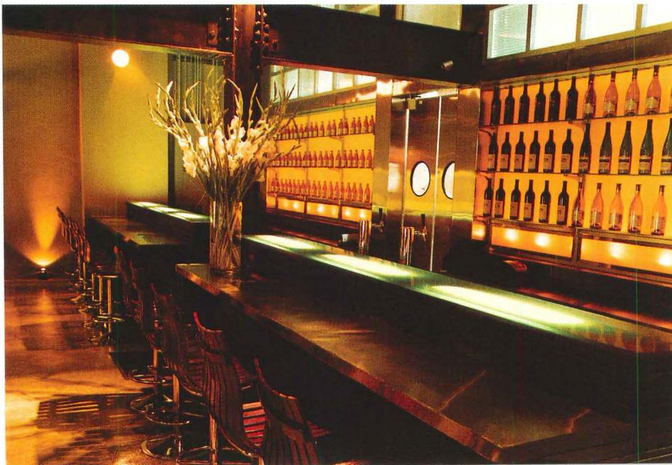
Vintage incandescent pendants and underwater halogens highlight the reflecting pool area (above). Linear fluorescents illuminate a bar top (left), with bottles backlit by PAR lamps fitted with yellow fil-
