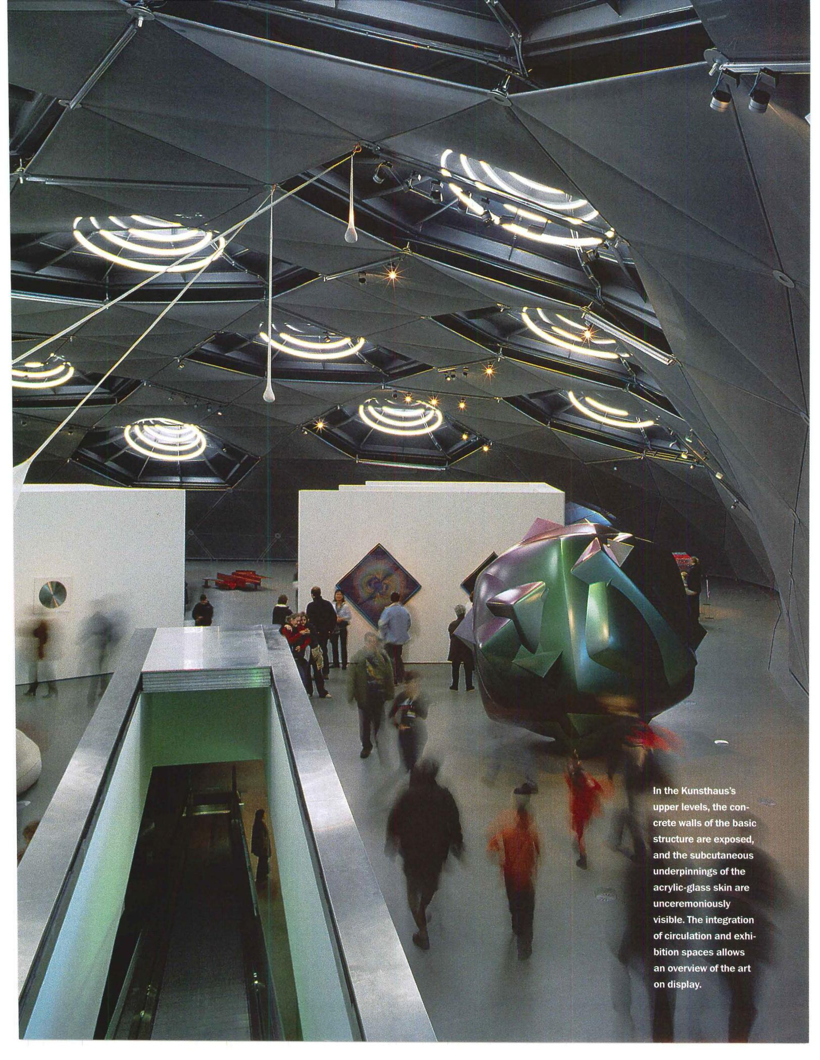
In the KunsthauS's upper levels, the concrete walls of the basic structure are exposed, and the subcutaneous underpinnings of the acrylic-glass skin are unceremoniously visible. The integration of circulation and exhibition spaces allows an overview of the art on display.
