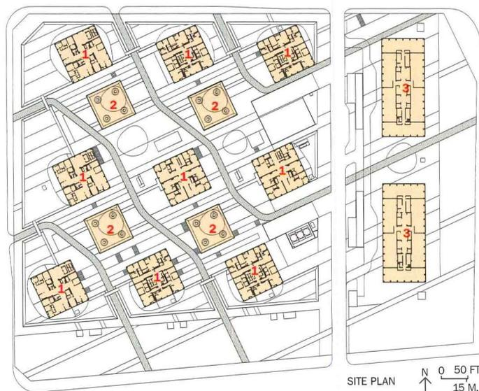
Yamamoto set the apartment towers (1) and mid-rise office blocks (2) within a checkerboard, then shifted the grid to respond to the Tonghui River (below). Two office wings (3) sit to the east, while future phases will be to the west (not shown).
