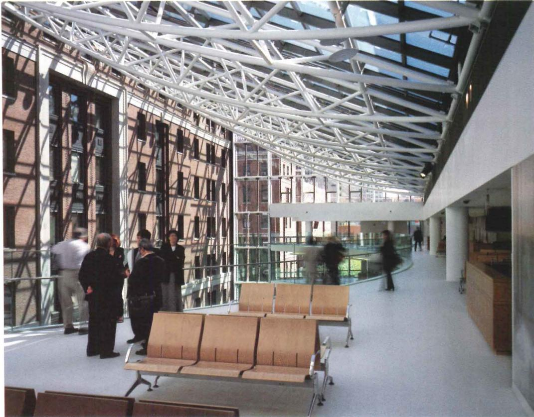
thanks to a sophisticated system of steel struts. The entire atrium is isolated from the ambulatory-care wing by a two-hour fire separation occurring along the spine between public and private program areas.
