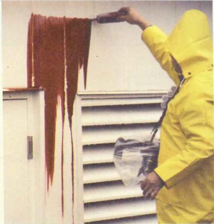
The owner of a former warehouse found evidence of water penetration in the building's mechanical space (left middle and bottom). Water testing (left) ruled out leaks in
