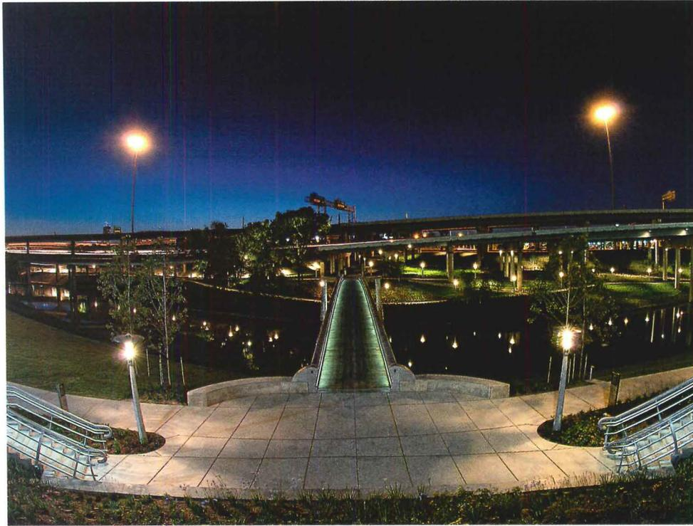
**Integral LEDs highlight pedestrian access; pole-mounted downlights illuminate paths; and stadium floods shine a blue wash on urban infrastructure.**
