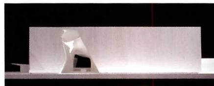
Moses's parting of the Red Sea. The curved surfaces of this negative space will comprise prefabricated modules of sandstone-mixed concrete, providing contrast to the rigid geometry of the tempered-glass building shell. The museum is scheduled to open in 2009. *David Sokol*
