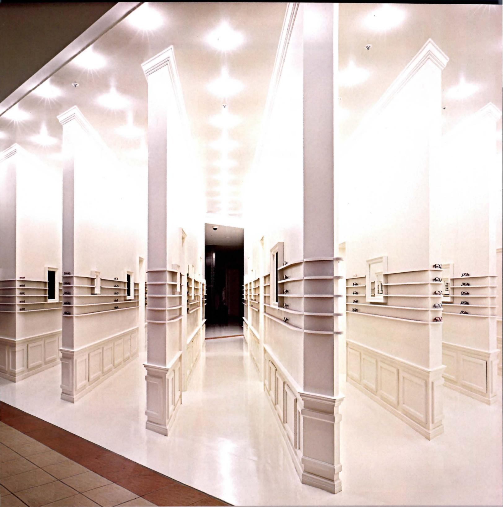
With acutely angled ends, the 8-inch-thick walls (above) create a forced perspective, aggrandizing their soaring appearance. The corridors' proportions—11 feet high and 3 feet wide—accentuate that effect. These slots of space are open-ended, enticing customers to slip in for a peek or a shortcut through the mall (opposite).
