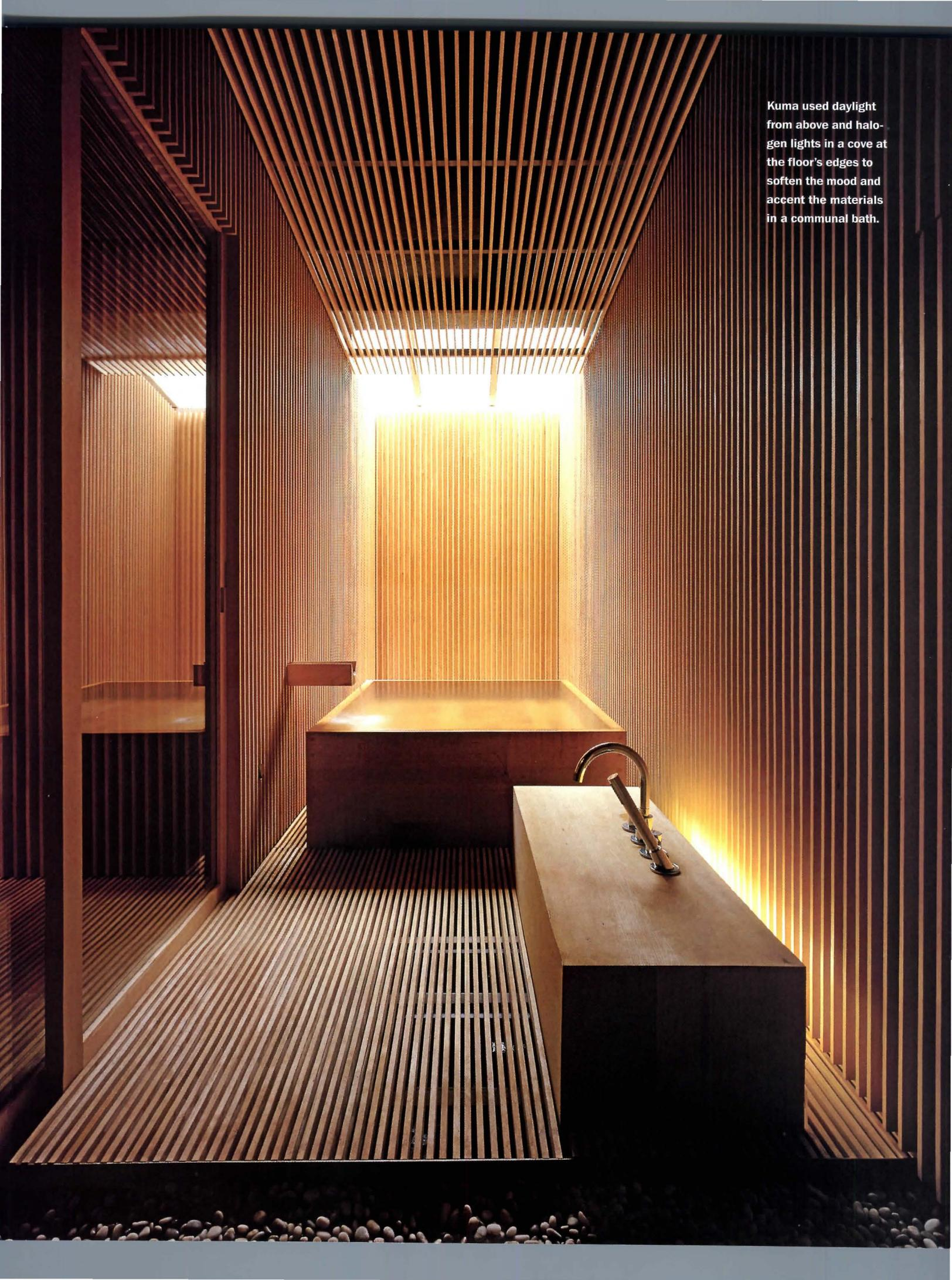
Kuma used daylight from above and halogen lights in a cove at the floor's edges to soften the mood and accent the materials in a communal bath.
