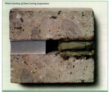
This photo shows the negligible impact of weathering on a silicone sealant (left) versus the degraded impact on an organic polyurethane sealant (right) after 3000 hours of accelerated weathering, which is equivalent to 3 to 6 years of actual outdoor weathering.
