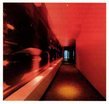
A high-resolution print of London's traffic runs along the 40-foot-long corridor wall, lit from below by a changing spectrum of LEDs set into a trough (left). tom LED-embedded wall washers—part of an off-the-shelf combined DJ and lighting system that includes a DMX-controlled light desk.
