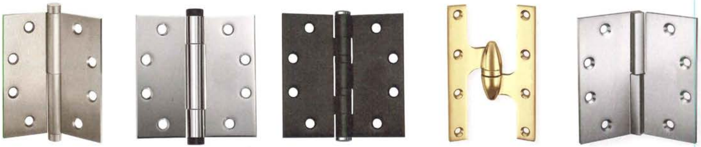
Some available types of door hinges include (left to right) two-knuckle hinge with decorative tips, three-knuckle hinge with decorative tips, five-knuckle hinge, olive-knuckle hinge, and a square barrel hinge.
