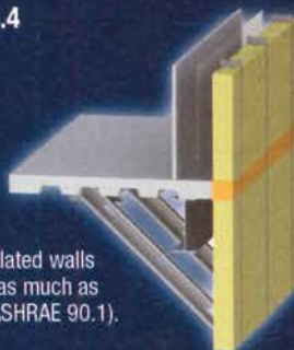
6" Traditional Stud Insulated Wall R-7.4
