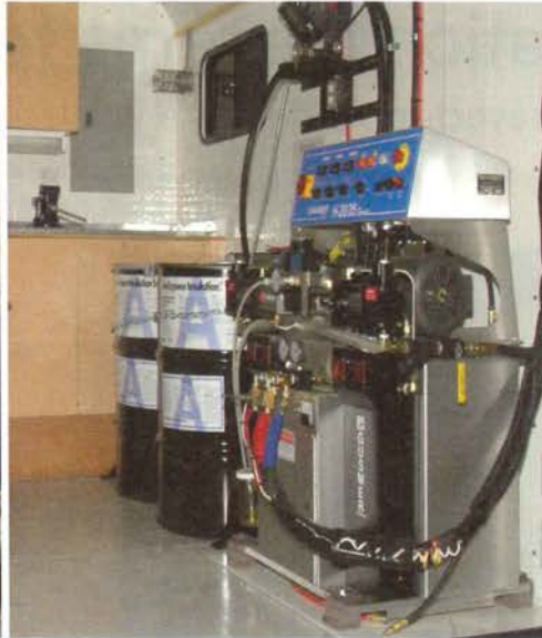
Spray foam insulation is mixed on site and applied using spray gun equipment appropriate to a particular manufacturer.
