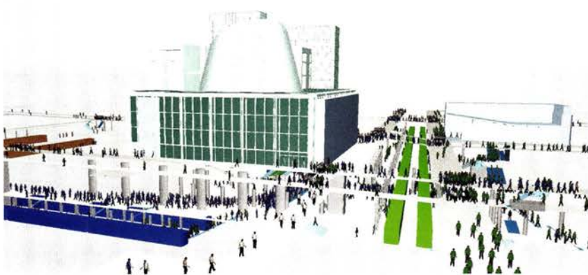
PEOPLE MOVER To understand how commuters would circulate through Fulton Center, Arup examined the complex with a crowd simulation tool developed in-house. The software populates the digital model with "agents," or virtual people.
