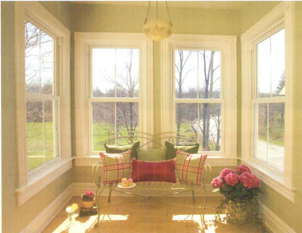
This historic bed and breakfast was retrofitted with airtight, double-glazed replacement windows with an Argon gas fill, low-emissivity (low-E) coatings, and vinyl frame construction that reduces thermal bridging and other through-wall energy loss.
