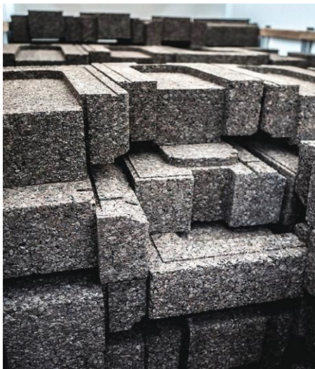
THE STRUCTURE , weather envelope, insulation, and interior finish (above) of the Cork House consist almost entirely of cork blocks (left) that are tongue-and-groove friction-fit together.
