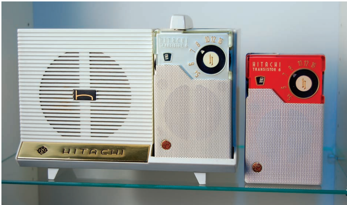
These 1959 Hitachi sets had an optional speaker box for a bigger sound at home. It plugs into the earphone jack on top of the radio.
