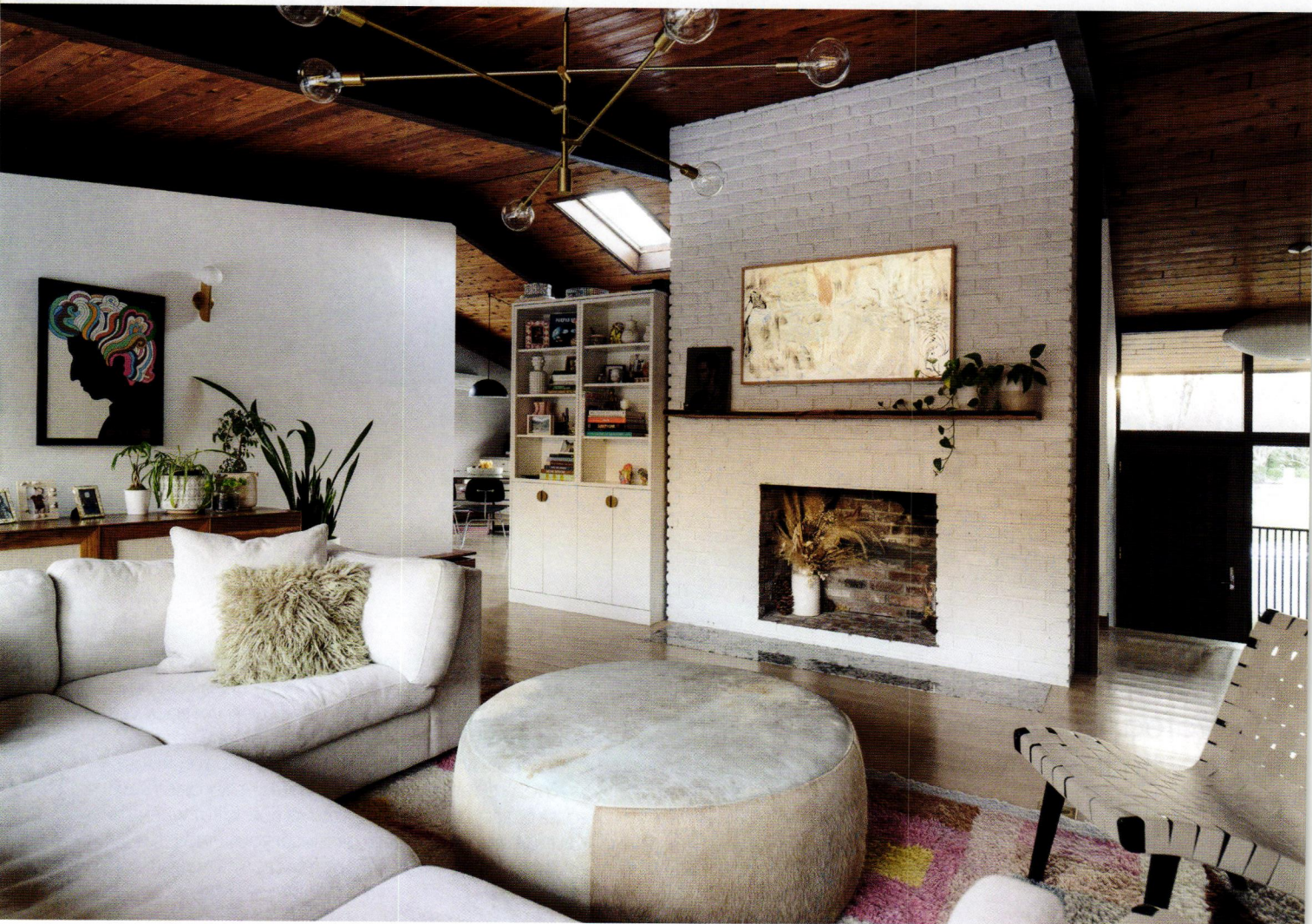
BELOW: THE ORIGINAL HEARTH OF THE FIREPLACE WAS A MASSIVE STONE SLAB ON TWO FEET OF BRICK THAT CAME UP TO ANKLE HEIGHT, WHICH WAS A NO-GO FOR A FAMILY OF TWO YOUNG GIRLS AND A THIRD ON THE WAY. SO THEY REMOVED THE STONE AND REPLACED IT WITH REMNANT STONE LAID IN FLUSH WITH THE HARDWOOD FLOORING. (DON'T WORRY ABOUT THE ORIGINAL STONE—IT FOUND NEW LIFE AS A STEP OUTSIDE THE ENTRYWAY!).
