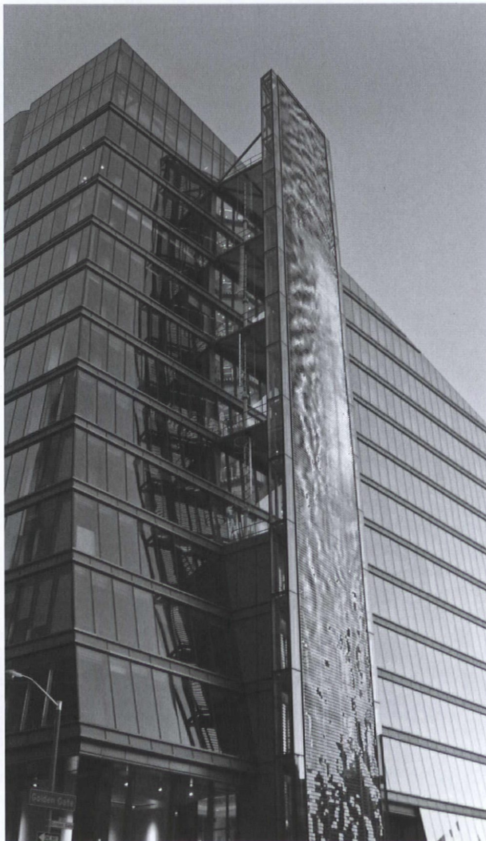
Above: Firefly , San Francisco, CA, 2012. A collaboration with KMD Architecture for the San Francisco Arts and Public Utilities commissions, Firefly reveals the wind moving around and through it. The hinged, polycarbonate panels swing with the patterns of the wind. By day, the work appears like rippling waves of glass. By night, the back-and-forth swinging of the panels triggers the flickering of tiny LED lights.
