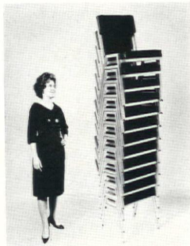
and may be stored as many as 12 high without danger of tipping. Frames of extruded aluminum are available in natural anodized finish or black anodized finish. A range of fabrics and supported vinyl upholstery is available. Seats are of 2-inch foam rubber, backs of one-inch foam rubber. Swivel glides are part of the design.
