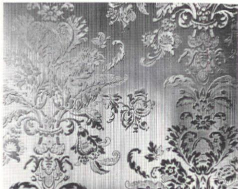
which is manufactured in The Netherlands by Balamundi Nederland N. V. In each of the 39 new patterns, the design is engraved permanently into the metallic surface of the material. The poly-vinyl-chloride surface is stainproof, easy to maintain, colorfast, odorless, and resistant to fire and dust. Shown here is one of the 39 patterns, Florence, a reproduction of ancient Italian damask that comes in orange, gold, silver, blue metallic, green gold, and rich gold.
