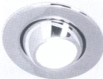
Fiberstar™ from Fiberstars provides aimable illumination without electricity, heat or ultraviolet radiation at the fixture. Each fixture has an output and quality of light approximating that of 35- to 50-watt MR series tungsten halogen lamps or 75- to 100-watt incandescent lamps. A remotely installed, shoebox-sized, U.L. listed Fiberstars illuminator provides the power and light source and can be conveniently placed in any space.
