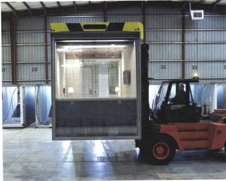
The 215 guestrooms are prefabricated in CitizenM's local factory (above). Separating out bathroom elements—a shower in one glass cylinder, a toilet in another dusted glass column, and a sink basin in a third Corian tube—allowed Concrete to maximize space in the 14-sq.-m. guestroom (below right). One section of the self-service food and beverage area of the lobby converts to a bar during evening hours (below left).
