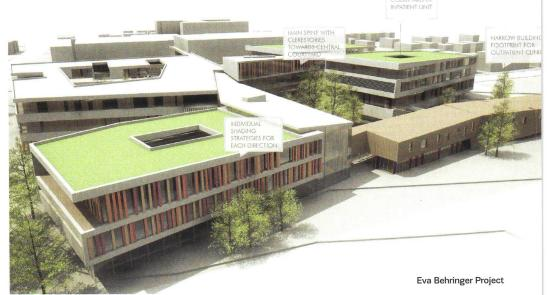
bed community hospital. The overall footprint is divided into smaller pavilions that create pockets of green space, maximize exterior views, and allow sun penetration from multiple angles. The central courtyard is fully accessible, and a main circulation spine connects all pavilions.
