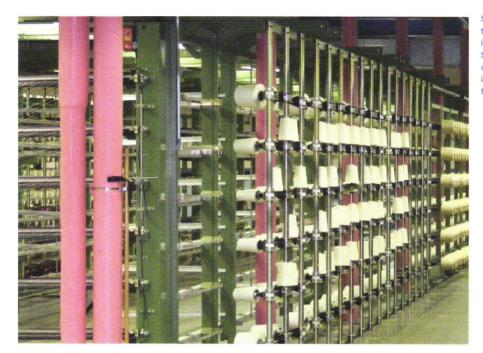
Sectional warping racks in the Sunbury Textile Mills in Sunbury, Pennsylvania. Sunbury produces as many as 2,000 patterns annually, including performance fabrics for Sunbrella and Crypton.
