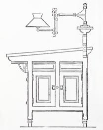
Model Drafting Tables.—Fig. 2.—End Elevation of Single Tables.—Scale, ½ Inch to the Foot.
