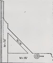
Door and Window Screens .- Fig. 4.-Manner of Bracing the Corners Employed by C. H. R.
