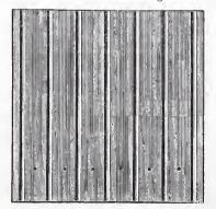
Metallic Shingles.—Fig. 3.—Corrugated Sheet Iron Siding, used for the Walls of Buildings in Connection with Metallic Shingles.
