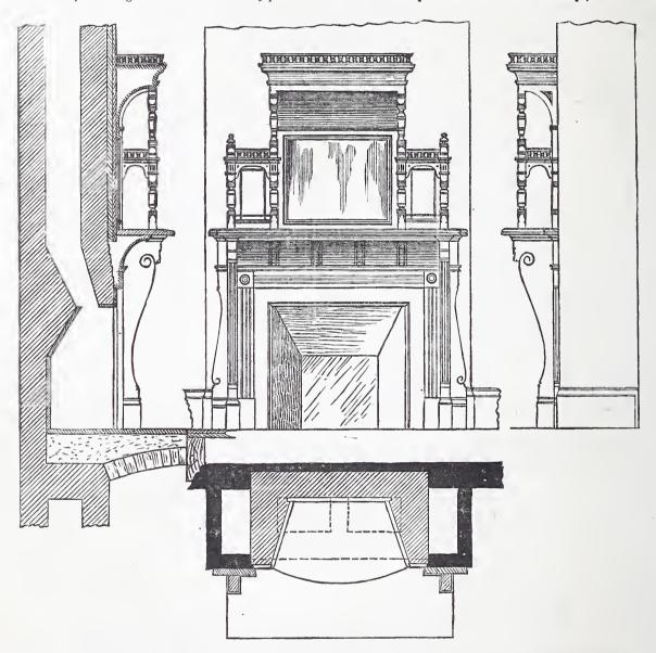
Dining Room Mantel and Mirror.—Fig. 2.—Section, Front Elevation, Side Elevation and Plan.—Scale, 1/2 Inch to the Foot.
