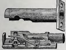
Recent Novelties.—Fig. 7.—Ives' Improved Door Bolt.—View Showing Working Parts.
