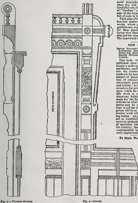
Design of Door, Door Trimming and Wainscoting .- Scale, 11/2 Inches to the Foot.
