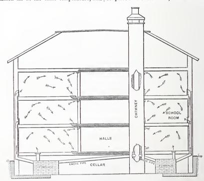
Ventilation.-Fig. 2.—Diagram shows Hot Air Pipe going up in the Outside Walls of the Building. Partition Walls are used for Same Purpose when Convenient. Several Exhaust Stacks are used in a Large Building.
