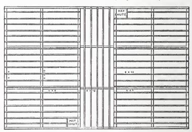
Framing a Bank Barn, -Fig. 6.-Plan of Floor Timbers.
