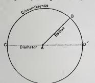
Stair Building .- Fig. 19 .- A Circle, with the Names of its Parts.
