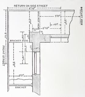
The Mechanics of Bracket Balconies .- Fig. 3 .- Plan of Balcony and Corner of Building .- Scale, 1/4 in. to Foot.
