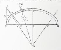
Semi-Ellipses.—Fig. 1.—Rule for Constructing the Figure from Three Centers .- Contributed by H. D. C.
