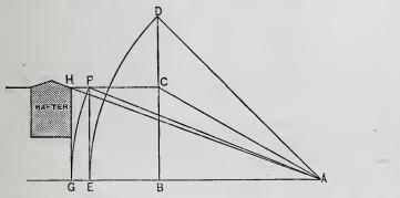
Backing Hip Rafters.--Fig. 5.—Application by G. H. H. of his Rule to Rafters of 7-Inch Rise to I Foot Run.
