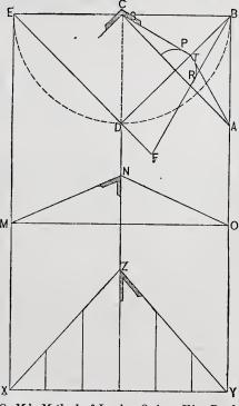
O. M.'s Method of Laying Out a Hip Roof.
