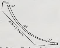
Hip Rafters.-Fig. 6.-Application of the Rules to Cove Hip Rafters.
