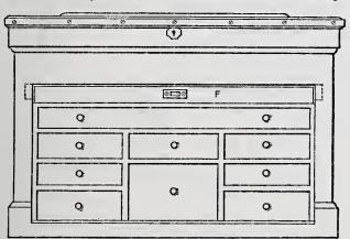
E. A. W.'s Chest.-Fig. 1.—Elevation of Chest, with Face of Drawers Exposed.— Scale, I Inch to the Foot.
