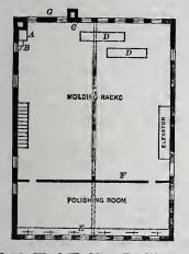
A Model Wood-Working Establishment. Fig. 6.-Fifth Floor. A, Water Closet. B, Sink. C, Iron Door to Shavings Chute. Benches. E, Bench with Polishing Lathes. F, Partition. G, Shavings Chute.
