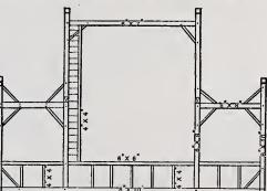
Framing of a Curb Roof Barn.-Fig. 5.-Construction of Middle Bents .- Scale, 1-16th Inch to the
