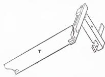
Wooden Turning Lathe.—Fig. 8.—Construction of Tool Rest in A. E. V.'s Lathe.
