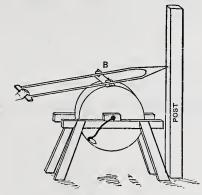
Jack for Grinding Tools.-Fig. 2.-Manner of Using the Jack.
