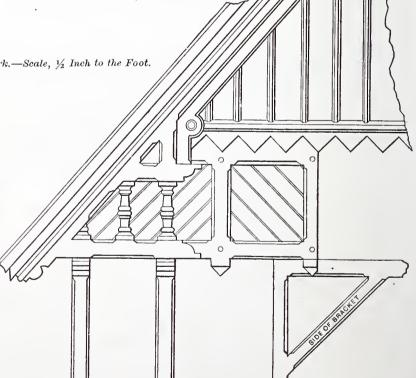
Frame Cottage.—Fig. 7.—Detail of Finish of Front Gable.—Scale, 1/2 Inch to the Foot.
