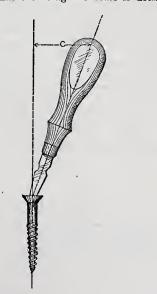
Advantages of Long and Short Screw Drivers. -Fig. 4.—Short Screw Driver with a Beveled Edge.
