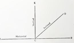
Stair Building.—Fig. 4.—Names of Lines with
