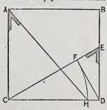
Rake Molding .- Fig. 2 .- Angles by which to Adjust Miter Box.
