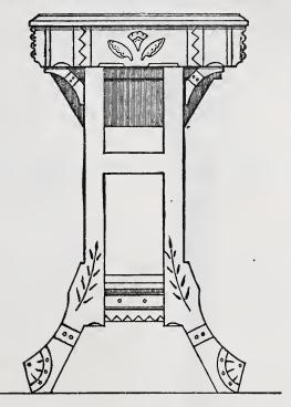
Ladies' Sewing Table.—Fig. 5.—End Elevation.— Scale, 11/2 Inches to the Foot.
