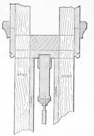
Construction of Sliding Doors.—Fig. 1.— Vertical Section through Top of Doors. —Letter from A. M.
