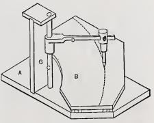
A Machine for Laying Out the Rail in Cylinder Stairs.
