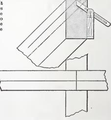
Backing Hip Rafters.—Fig. 4.—Hip Rafters Cut to Butt against each other. Bevel set to the Run, Rise and Length of Hip Rafters.
