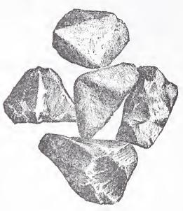
"Sharp" Sand and Quicksand.—Fig. 2.—Grains of Good Building Sand Highly Magnified.—From a Photograph.
