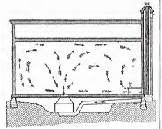
Church Ventilation.—Fig. 1.—Longitudinal Section through a Church 50 by 60 Feet. with 25-Foot Ceiling.
