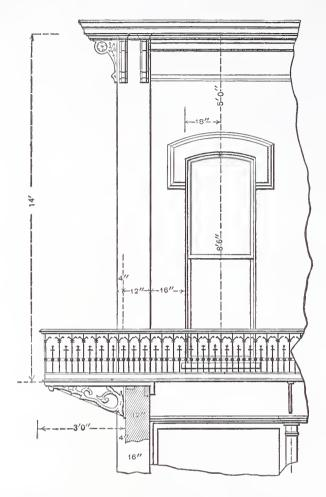
The Mechanics of Bracket Balconies.-Fig. 1.-Elevation of Corner of Second Story of Store Building .- Scale, 1/4 Inch to the Foot.
