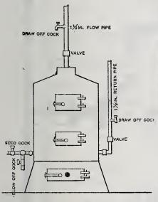
Hot Water Heating.—Fig. 1.—Diagram of Boiler, showing Valves, Draw-off Cocks, &c.
