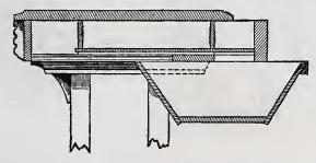
Ladies' Sewing Table.-Fig. 4.-Vertical Section, showing Construction and Arrangement of Drawers.—Scale, 11/2 Inches to the Foot.
