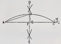
Stair Building.-Fig. 47.-Drawing a Straight Line Approximately Equal to a Given Arc without Having Recourse to the
