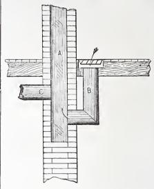
Heating and Ventilation.—Fig. 7.—Ventilateating and ventilation.—Fig. 7.—Ventilat-ing a Church by Connecting an Opening in the Floor with the Main Chimney Flue, Making the Connection Below the En-trance of the Furnace Pipe. A, Chimney Flue. B, Ventilation Tube. C, Position of Furnace Pipe.
