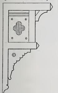
Frame Church.—Fig. 6.—Detail of Brackets to Door Hoods .- Scale, 1/2 Inch to the
