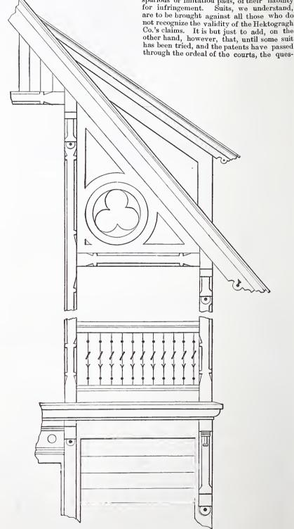
A Frame Dwelling.—Fig. 7.—Detail of Work at Sides of Front Gable and of Balcony.— Scale, 1/2 Inch to the Foot.
