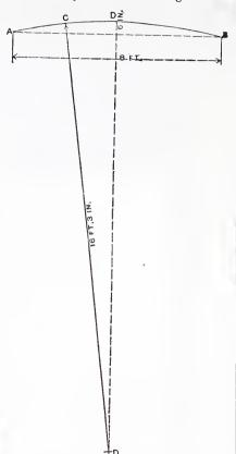
Determining Radius, Length of Chord and Rise bzing Given.—Fig. 1.—Rule Presented by C. O.
