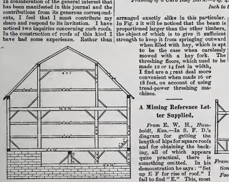
Framing of a Curb Roof Barn.—Fig. 2.—Construction of End Bents.—Scale, 1-16th Inch to the Foot.
