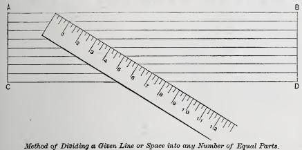
Method of Dividing a Given Line or Space into any Number of Equal Parts.
