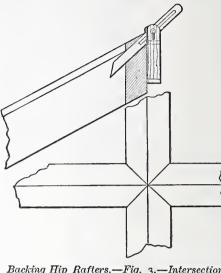
of Four Hips. The Down Bevel for Top of Common Rafter Applied to the End of Hip Rafter.
