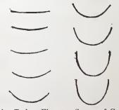
Carving Tools.—Fig. 12.—Sweeps of Gouges. ments are so easy, it seems strange that errors of this kind are allowed to go so long unchallenged as is sometimes the case.
