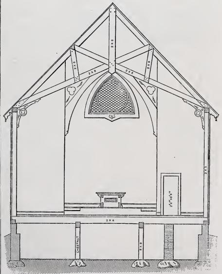
Frame Church.—Fig. 7.—Transverse Section through Audience Room.—Scale, 1/3 Inch to the Foot.
