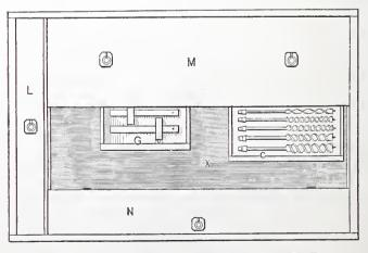
X. Y. Z.'s Tool Chest.-Fig. 4.—Horizontal Section near Top; M, Top of Drawer Case; N, Lid to Saw Rack; X, Bottom of Chest; G and C, Drawers, designated by like letters in Fig. 2, partly drawn out; L, Lid to Chiscl Rack.
