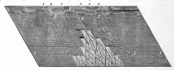
Metallic Shingles.—Fig 2 - Diagram Illustrating the Method of Laying the Shingles on a Roof.
