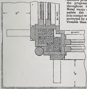
Suburban House.—Fig. 13.—Detail of Corner of Bay Window.—Scale, I 1/2 Inch to the Foot.
