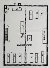
A Model Wood-Working Establishment. Fig. 5.—Fourth Floor. A, Sink. B, Water Closet. C, Benches. D, Heater for Cauls. -Fourth Floor. A, Sink. B, Water E, Steam Glue Pot. F, Saw Bench. G, Chute for Shavings. E, Iron Door Connecting with Shavings Chute.
