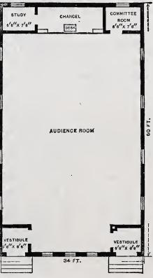
Frame Church.-Fig. 3.-Plan. I-16 Inch to the Foot.
