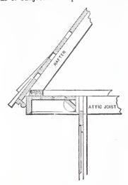
Suburban House.—Fig. 16.—Detail of Roof of Bay.—Scale, 1/2 Inch to the Foot.
