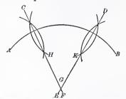
Stair Building.—Fig. 37.—To Find the Center by which a Given Arc is Struck.
