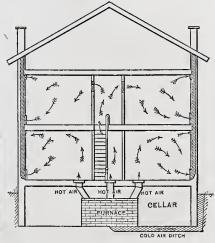
$Ventilation.-Fig.\ 5.-Section\ of\ House,\ show$ ing Method of Heating and Ventilating Sleeping Rooms in Upper Story. The ordinary arrangement of the Flues is Utilized to obtain Ventilation and Heating for the Rooms both above and below. Greatly inferior to the Plan shown in Fig. 1.
