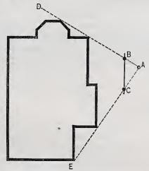
An Easy Way to Level the Bottom of a Cellar.
