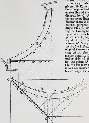
Hip Rafters for Mansard Roofs.—Fig. 2.—Method Recommended by A. M.
