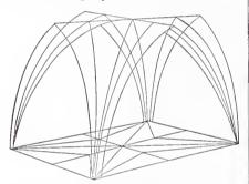
Vaults and Groins,-Fig. 2.-Illustration of Plain Ribbed Vaulting, the Vaults being of Equal Hight.
