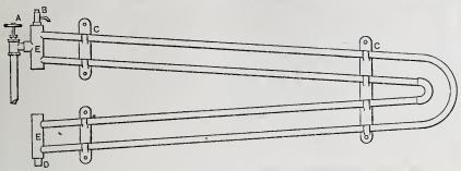
Hot Water Heating .- Fig. 8 .- Circulation Coil with Branch Tees or Headers; Suitable for Running Long Distances Around Walls .-- A, Valve. B, Air Vent. C, Hook Plates. D, Return Pipe. E Headers. F, Flow Pipe.
