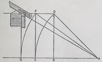
Backing Hip Rafters.—Fig. 6.—Application of Rule to Rafters Having I Foot Rise to I Foot Run.
