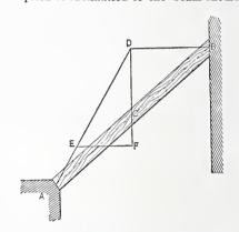
Roof and Bridge Trusses .- Fig. 4.- Determining the Strains upon an Inclined Bea Loaded Uniformly along its Whole Length.
