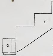
Straight Flight of Stairs with Cylinder .-Fig. 12.—Elevation of Front String, terminated by a Cylinder at the Top.
