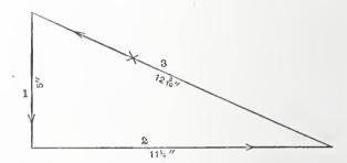
The Mechanics of Bracket Balconies.-Fig. 4.-Diagram of Strains.—Scale, I Inch to 1000 pounds.
