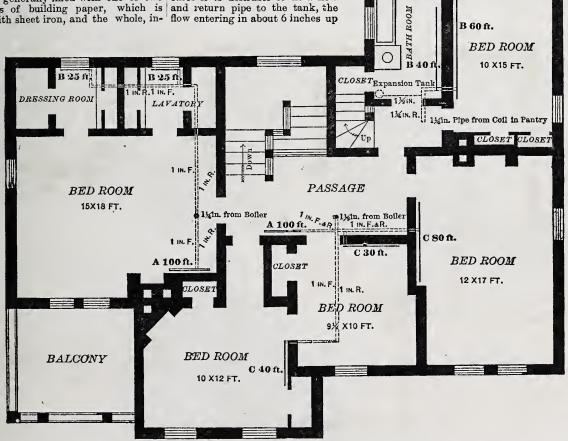
Hot Water Heating.—Fig. 9.—Second Floor Plan of Suburban Residence, Showing Position of Fixtures, Runs of Pipe, &c.— Scale, 1/8 Inch to the Foot.
