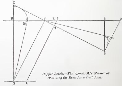
at right angles to h draw h e; then we bave a triangle F h e. Similar to the triangle F H E draw h k, which corresponds to H K. Now, as K E represents how much the but joint is from being a square cut, so will k e on the larger scale represent the same thing; therefore, taking F h as a square cut, and setting off h a equal to k e, and connecting
