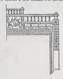
Designs for Interior Woodwork.-Fig. 3.-Alternative Design for Top of Pier Glass Frame. -- Scale, 3/4 Inch to the Foot.
