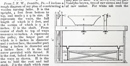
Wood Turning Lathe .- Fig. 2. - Side Elevation.
