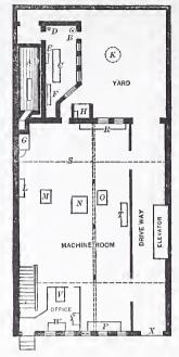
Model Wood Working Establishment. -First Floor. A, Lowe Boiler. B, teater. C, Buckeye Automatic En-Fig. 2.-Lowe Heater. C, Buckeye Automatic Engine. D, Engineer's Closet. E, Worthington Duplex Pump. F, Fly Wheel. G, Water Closet. H, Shavings Chute. K, Cistern or Cesspool. L, Jointer. M and N, Molding Machines. O, Pony Planer. P, Bench. R, Swing Cut-Off Saw and Bench. S S, Line Shafting. T, Saw. V Y, Desks in Office. W, Drawing Table. X, Gate to Drive Way. Lowe Heater.
