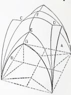
Vaults and Groins .- Fig. 6.- Example of Groining in which Intersecting Vaults are of Unequal Hight.
