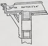
Cheap Frame House .- Fig. 7 .- Section through Piazza Cornice .-Scale, 3/4 Inch to the Foot.
