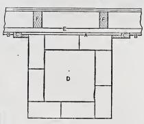
A. Old Clapboards. B. New Clapboards. C. Rebated Strip, put over Ends of Old Boards.D. Chimney. E. Boarding. F. Studding.
