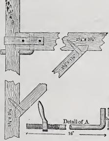
Staging Backets.—Fig. 2.—Details of Construction of Brackets shown in Fig. 1.
