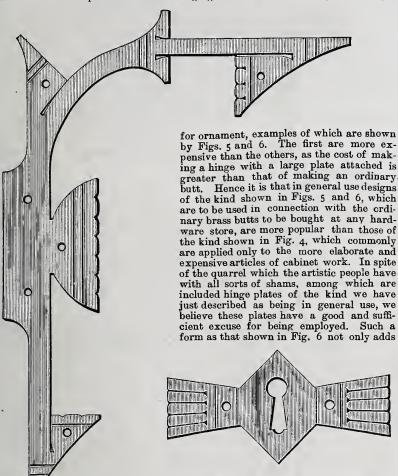
Cabinet Hardware. - Fig. 6. - Antique Corner Hinge-Plate (Half Size).
