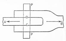
The Shearing Strength of American Woods. The Method of Experimentation Pursued by Mr. Trautwine. B, Iron Holder. PP, Pin Passing through the Parts in a Cylindrical Hole. Arrows denote Direction of Strain.
