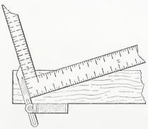
Backing Hip Rafters.—Fig. o.—Method of Setting the Bevel as Originally set Forth by G. H. H.
