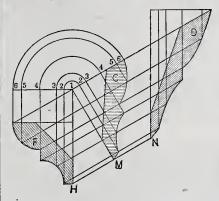
Rake Molding .- Fig. 1. - Manner of Developing the Shape.
