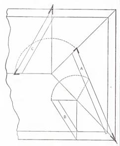
Hip Rafters.—Fig. 1.—Plan of Roof.
