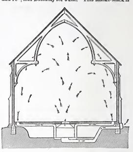
Church Ventilation .- Fig. 4.- Transverse Section through Church 70 by 100 Feet, 40-Foot Ceiling.
