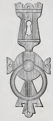
Cabinet Hardware.—Fig. 9.—Ring Handle for Cabinet or Drawer, with Key Plate and Striking Plate (Full Size).
