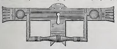
Cabinet Hardware .- Fig. 7 .- Drawer or Cabinet Handle, with Key Plate and Striking Plate (Full Size).
