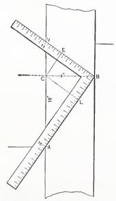
Hopper Bevels.—Fig. 2.—E. W. C.'s Rule.— Drafting the Hopper by use of the Square.
