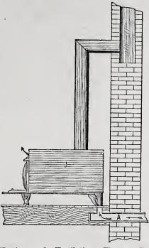
Heating and Ventilation.—Fig. 3.—The Same Principles Applied to Box Stoves, the Jacket Enveloping the Entire Stove except the Front. A, Supply of Outdoor Air. J, Jacket. Arrows show the Division of the Chargest. Air. J, Jacket. Arr rection of the Current.
