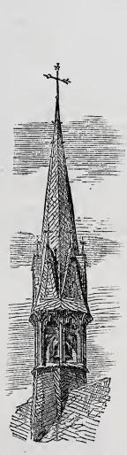
Fig. 2.—Bell Turret from Cassel, 14th Century. Pinnacle and Base Covered with Small Slates.
