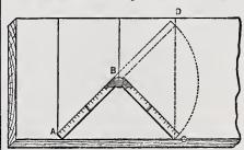
Method of Squaring a Board or Piece of Timber by Use of Pocket Rule.
