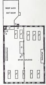
Model Wood-Working Establishment .-Fig. 4.—Third Floor. A, Sink. B, Water Closet. C, Hardware Closet. D, Heater for Cauls. E, Steam Glue Pots. F, Benches. G, Shavings Chute. H, Iron Door Communicating with Shavings Chute.
