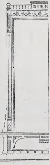
Designs for Interior Woodwork.-Fig. 2. Pier Glass Frame. -- Scale, 3/4 Inch to the Foot.
