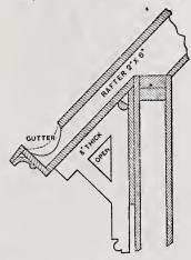
Cheap Frame House,-Fig. 8.-Section of Main Cornice.—Scale, 3/4 Inch to the Foot.
