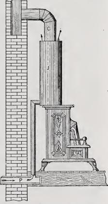
Heating and Ventilation.—Fig. 4.—Heating Outdoor Air by Means of a Jacket Around the Stove Pipe. C, Stove Pipe. J, Jacket. the Stove Pipe. C, Stove P, Supply of Outside Air.
