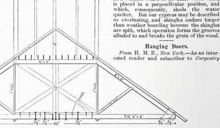
Roof Trusses.—Fig. 2.—Truss in Church Roof.—Sketch Accompanying Letter from W. A. W.
