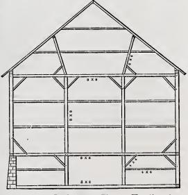
Framing a Bank Barn.—Fig. 3.—Elevation of End Bents.
