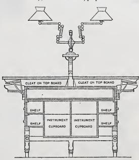
Model Drafting Tables .- Fig. 4.-Cross Section Through End of Double Table.—Scale, 1/2 Inch to the Foot.
