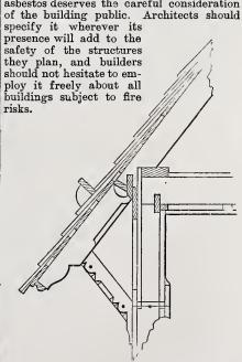
Suburban House.—Fig. 15.—Detail of Eaves and Cornice.—Scale, 1/2 Inch to the Foot.
