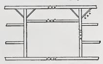
Framing of a Curb Roof Barn,-Fig. 3. Construction of Sides .- Scale, 1-16th Inch to the Foot.
