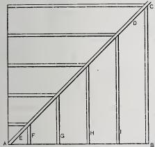
Determining the Lengths of Jack Rafters.
