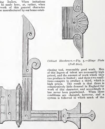
Cabinet Hardware. - Fig. 4. - Corner Hinge Plate, with Hinge Attached (Half Size).
