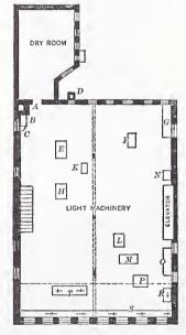
Model Wood-Working Establishment.— Fig. 3.—Second Floor. A, Door to Dry Room. B, Water Closet. C, Sink. D, Shavings Chute. E, Pony Planer. F, Band Saw. G, Bench. H, Saw Bench. K, Variety Machine. L, Grindstone. M, Boring Machine and Miter Saw. N, Machinery for Running Elevator. O, Fluting Machine. P, Sandpaper Ma-chine. R, Lathe for Turning Circles. S and T, Benches with Turning Lathes.
