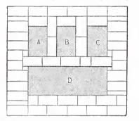
eating and Ventilation.—Fig. 5.—Construction of Chimney for both Smoke and Heating and Ventilation. D, Smoke Flue. A, Ven-tilation Flue for First Story. B, Ventila-tion Flue for Second Story. O, Ventila-tion Flue for Third Story.
