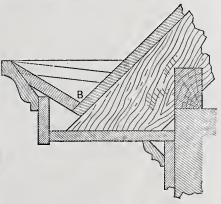
A. N. H.'s Construction of Gutter.
