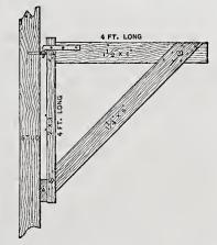
Staging Brackets.—Fig. 3.—T. J. L.'s Plan of Construction.
