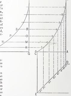
Hip Rafters for Mansard Roofs.—Fig. 5. Diagram Illustratiny Principles.
