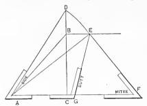
Hopper Bevels.—Fig. 1.—W. H. C.'s Rule Applied to Hoppers all Sides of which Flare Equally.
