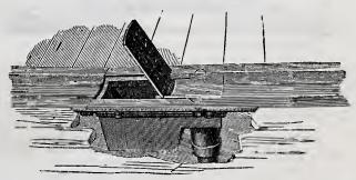
Stable Furniture.—Fig. 9.—Stall Gutter Plate, showing Connection with Stench Trap.
