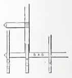
Design for Well House.—Fig. 4.—Plan of Roof Framing at Corner.—Scale, 1/4 Inch to the Foot.
