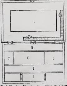
view of chest, showing two drawers for bench planes, and whatever a carpenter wishes to put in them. Fig. 6 is a top view of the chest. A is a saw-rack, B and B are for molding planes; C D is for oil stone, gauges, &c.; E for bits. Now, this design
