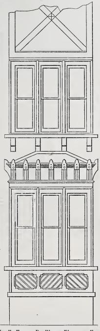
Small Frame Dwelling.—Fig. 9.—Front View of Bay and Chamber Windows. Scale, ¼ Inch to the Foot.
