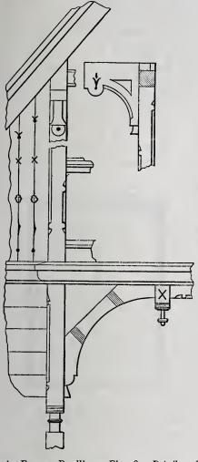
Frame Dwelling.-Fig. 8.-Details of Front Gable and Balcony .- Scale, 1/2 Inch to the Foot.
