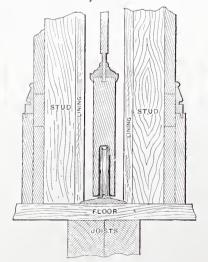
Construction of Sliding Doors.—Fig. 3.— Vertical Section through Bottom of Doors. —Letter from A. M.
