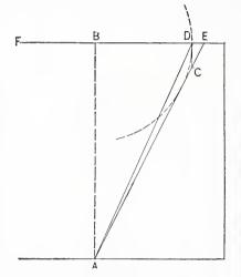
Hopper Bevels.—Fig. 3.—A. M.'s Amendment to the Rule for Obtaining the Bevels for Joints.
