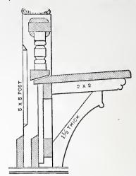
Design for Well House.—Fig. 3.—Section through Seat.—Scale, I Inch to the Foot.
