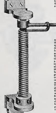
Novelties .-- Fig. 10.-- Door Spring Adapted to use in Steam Fire Engine Houses .- Scale, about 1/3 Full Size.
