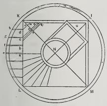
Groins, Pendentives and Niches .- Fig. 13. Method of Finding the Springing Lines of the Pendentives, the Section in a Vertical Planc being Given.
