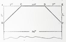
Making a Square Stick Octagonal.—Fig. 4.-Part Section Through a Stick 24 Inches Square after Shaping.
