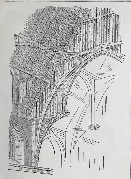
Ancient Hammer-Beam Roofs.—Fig. 6.—Roof of Westminster Hall, built A. D. 1397.— Span, 68 Feet .- Total Length, 238 Feet 8 Inches.
