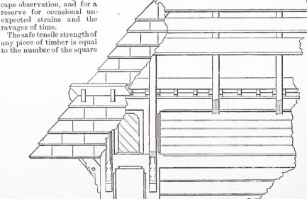
Suburban House.—Fig. 17.—Detail of Roof Construction.—Scale, 1/2 Inch to the Foot.
