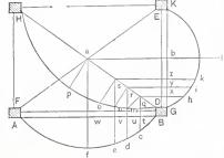
Groins, Pendentives and Niches.—Fig. 2.— Method of Describing the Sides of a Groin with Arches of the Same Hight.
