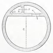
Pure Water.—Fig. 2.—Horizontal Section through Cistern near Bottom, Showing Con partments in Filter.—Letter from G. W. B.
