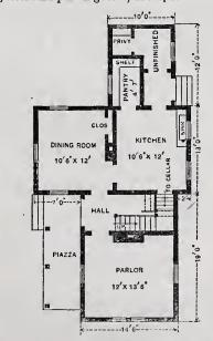
Cheap Frame House.—Fig. 2.—First Floor Plan .- Scale, 1-16th Inch to the Foot.
