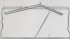
Hopper Bevels .-- Fig. 5.-- E. W. C.'s Rule .-- Manner of Placing the Square for a Miter Joint .
