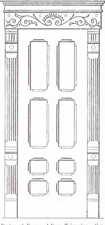
Design of Door and Door Trimming.—Contributed by W. T.—Scale, ½ Inch to the Ft.
