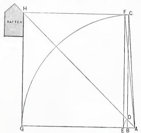
Backing Hip Rafters.—Fig. 8.—Diagram showing Close Approach to Perpendicular. Backing of the Rafter is at an Angle of almost 45 Degrees from the Side of the Rafter.
