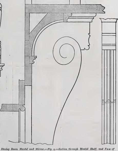
Pilaster.—Scale, 3 Inches to the Foot.
