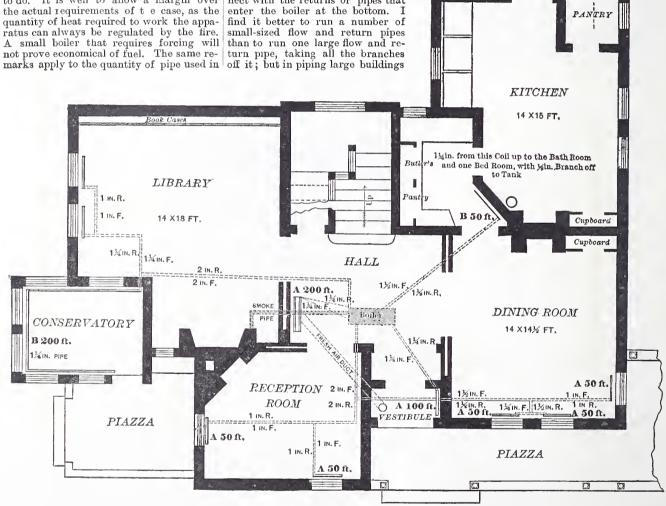
Hot Water Heating .- Fig. 7. - First Floor Plan of Suburban Residence, Showing Position of Fixtures, Runs of Pipes, &c. Scale, 1/8 Inch to the Foot.
