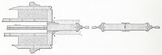
Construction of Sliding Doors.—Fig. 2.—Horizontal Section through Stiles, Jambs, &c.—Letter from A. M.
