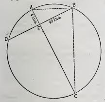
Determining the Radius of a Circle, Length of Chord and Rise being Given.
