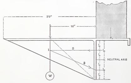
The Mechanics of Bracket Balconies.-Fig. 2.-Diagram of Opposing Forces, showing position of Concentrated Load, location of Neutral Axis, &c.—Scale, I Inch to the Foot.
