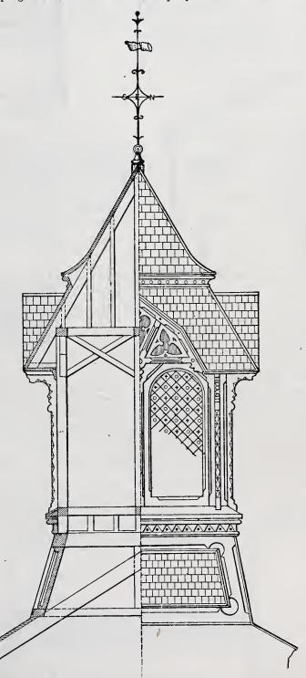
Design for Cupola, by H. N. T.—Scale, 1/4 Inch to the Foot.
