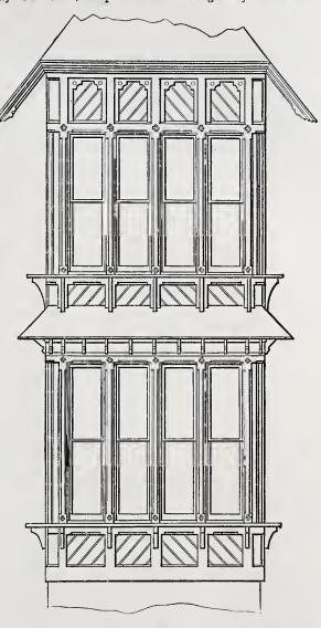
Suburban House.-Fig. 14.-Elevation of Bay Window.-Scale, 1/4 Inch to the Foot.
