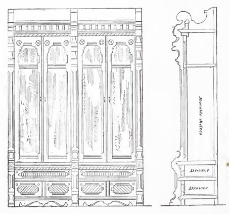
Design for Book Case.—Fig. 1.—Elevation and Section.—Scale, 1/2 Inch to the Foot.
