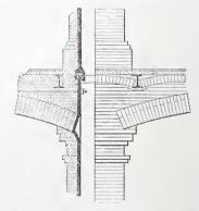
Fire-Proof Construction.—Fig. 9.—Cast-iron Columns Protected by 4½ Inches of Brick. Instead of Girders, Brick Arches are Sprung Between Columns, for Supporting the Floors.
