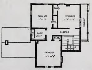
A Frame Dwelling.-Fig. 5.-Second Floor Plan.-Scale, 1-16th Inch to the Foot.
