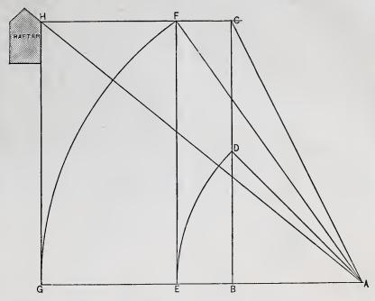
Backing Hip Rafters.—Fig. 7.—Application of Rule to Rafters Having 2 Feet Rise to I Foot Run.
