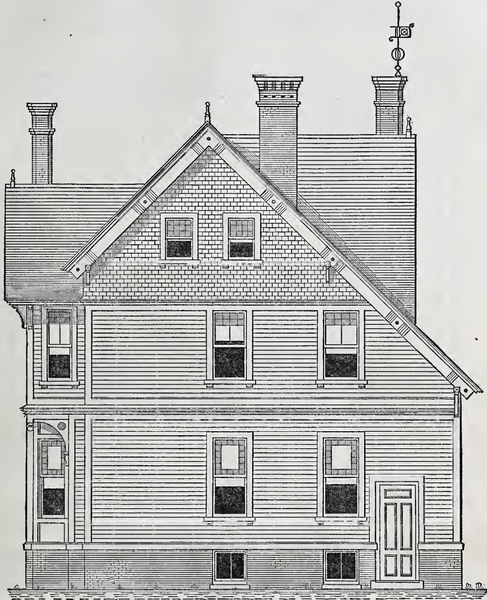
An English Cottage.—Fig. 8.—Rear Elevation.—Scale, 1/8 Inch to the Foot.
