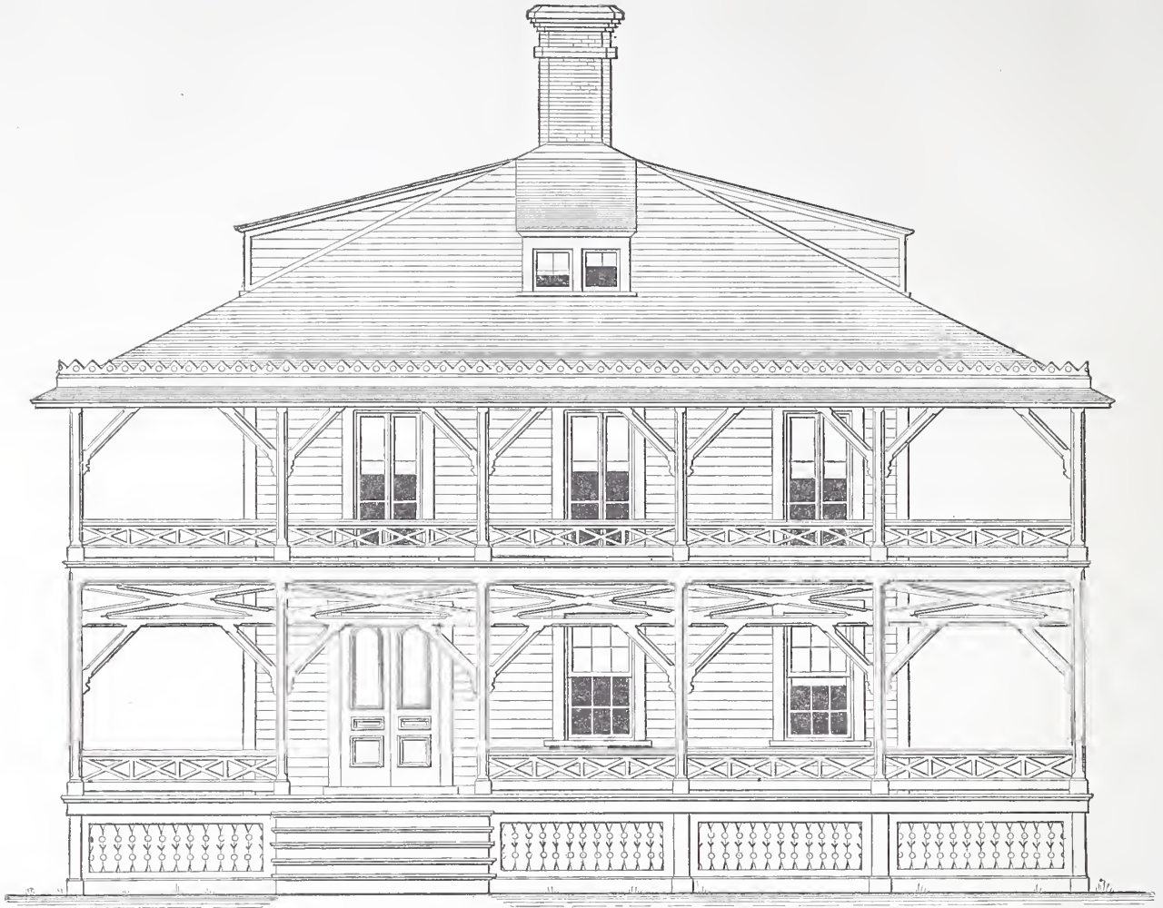
Southern Residence.—Fig. 1.—Front Elevation of House.—Scale, \frac{1}{8} Inch to the Foot.—A. Chamberlain, Architect, New Rochelle, N. Y.
