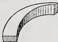
Stair Railing.—Fig. 7.—Perspective View of a Wreath Piece or Twist.
