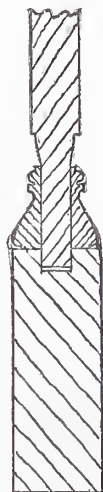
Design for a Village School-House.—Fig. 8. —Section through Stile of Entrance Doors.—Scale, 3 Inches to the Foot.
