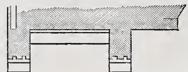
Fig. 22.—Horizontal Section through Supports to Mantel, Design B.—Scale, 1 1/2 Inches to the Foot.
