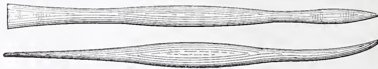
Lessons in Carving.—Fig. 3.—A Chisel-Shaped Tool with Bent Point.
