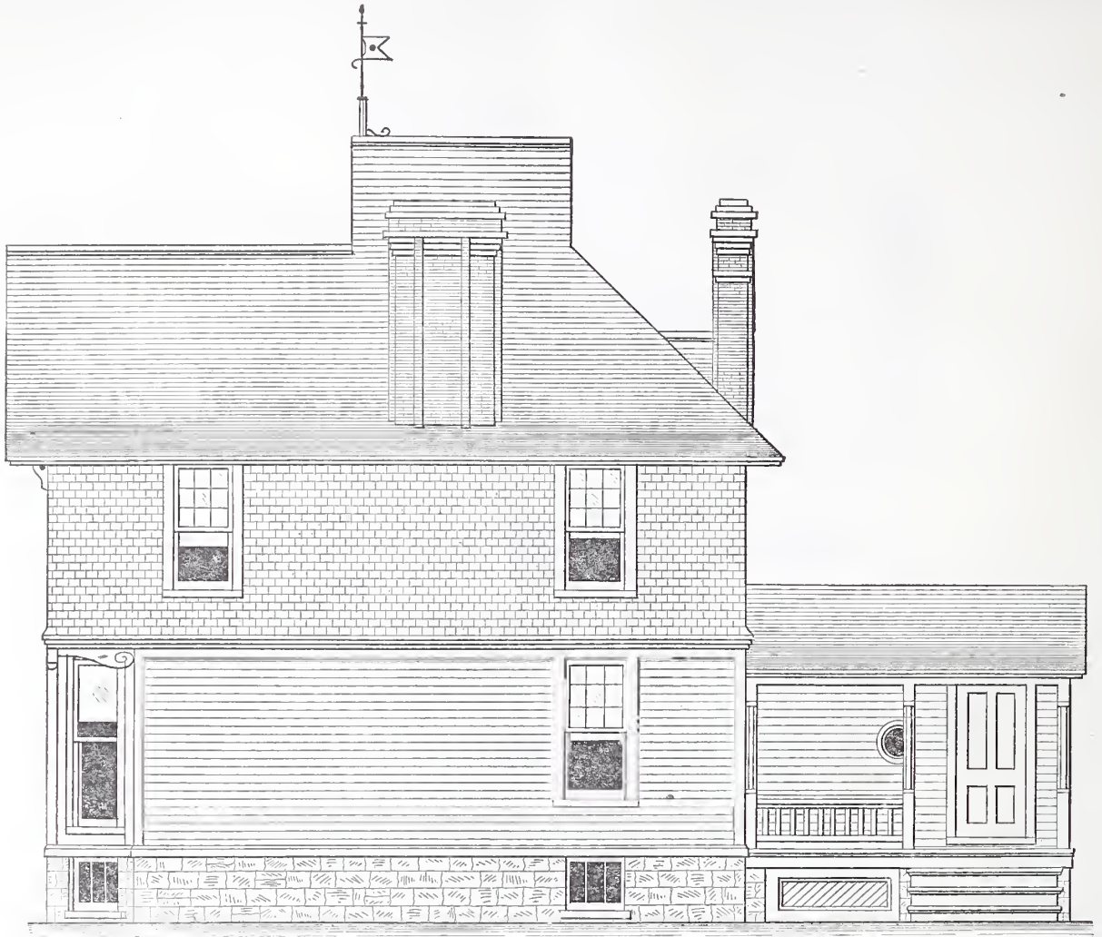
$3500 Dwelling Houses.—First Prize Design.—Fig. 6.—Side Elevation (Left).—Scale, \frac{1}{8} Inch to the Foot.
