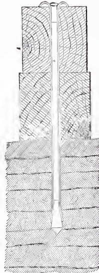
Anchoring Timbers to a Rock Foundation.
