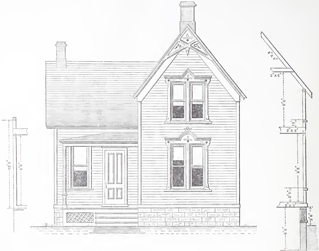
Cheap Frame House.—Fig. 1.—Front Elevation and Sections of House.—Designed by Elias Ayars, Hornellsville, N. Y., and Erected at a Cost of $700.—Scale, 1/8 Inch to the Foot. (See description on next page.)
