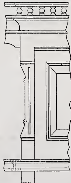
Fig. 5.—Finish Above Mantel.—Design B.—Scale, 1 1/2 Inches to the Foot.
