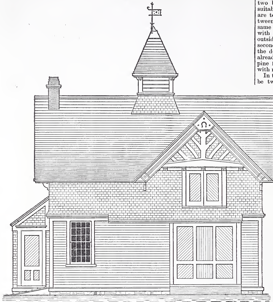
Design for Frame Stable.—Fig. 2.—Front Elevation.—Scale, 1/8 Inch to the Foot.
