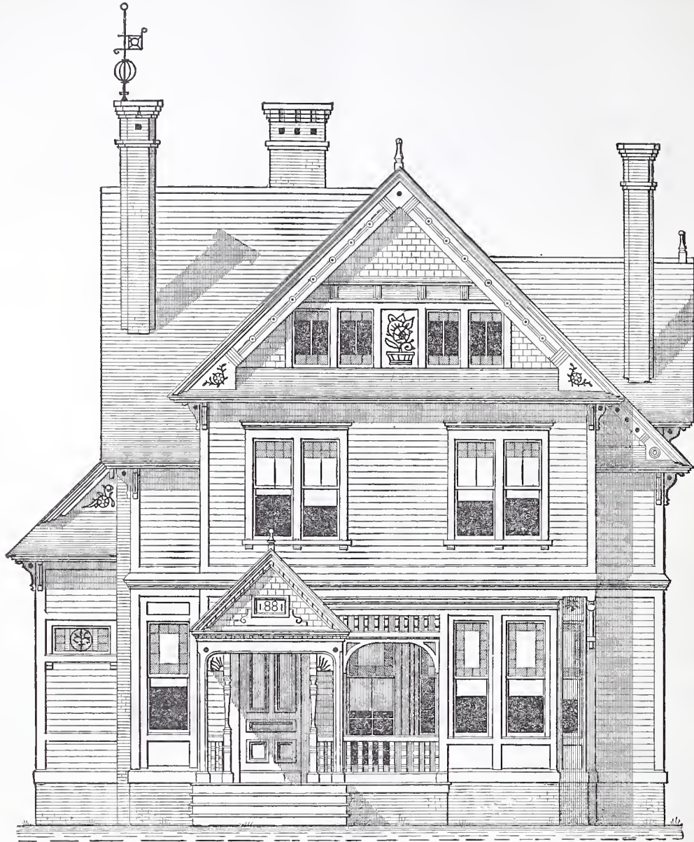
An English Cottage.—Fig. 2.—Front Elevation.—Scale, 1/8 Inch to the Foot.
