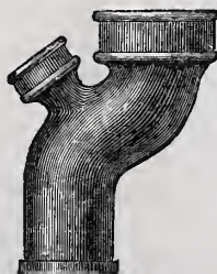
Fig. 20.—An Offset with an Inlet at the Side.
