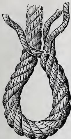
Fig. 41.—First Step in an Eye Splice in a Three Stranded Rope.
