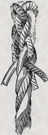
Fig. 18.—The Finished End. Ends of Strands are Tucked Under.
