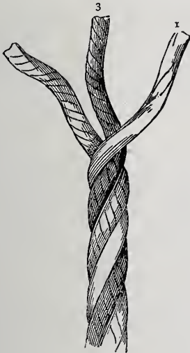
Fig. 12.—Rope Unlaied Ready for Securing the End.
