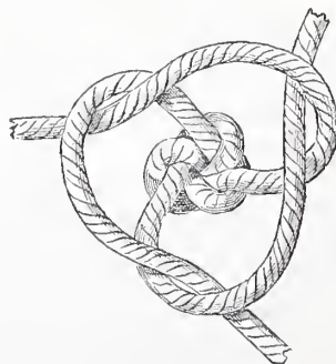
Fig. 23.—Top View of a Wall Knot Crowned by Interlacing the Ends before Jamming Down.
