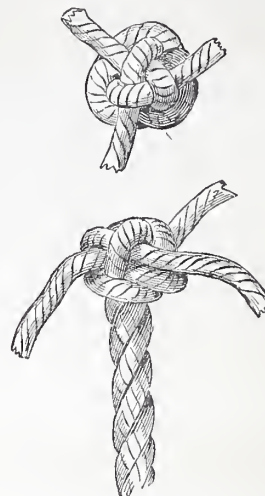
Fig. 24.—Top and Side View of a Wall Knot Crowned by Interlacing the Ends after Completion.
