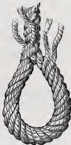
Fig. 46.—Commencing an Eye Splice in a Four Stranded Rope.
