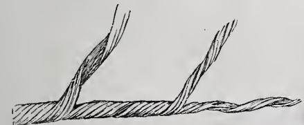
Fig. 32.—A Strand Tapered before being Struck.
