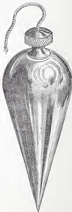
Fig. 3.—Plumb Bob Removed from the Case, showing the General Shape of the Article.
