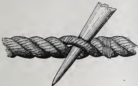
Fig. 29.—First Step Toward Interlacing or Weaving the Strand.
