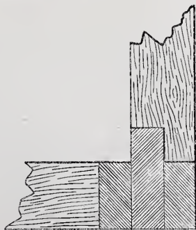
Corners of Frame Buildings.—Fig. 1.—Construction of an Outside Angle.
