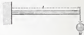
Fig. 12.—Beam Fixed at one End and Loaded at the Other.
