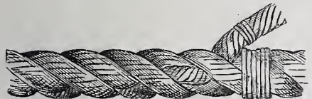
Fig. 31.—A Strand Interwoven with the Strands of a Rope.
