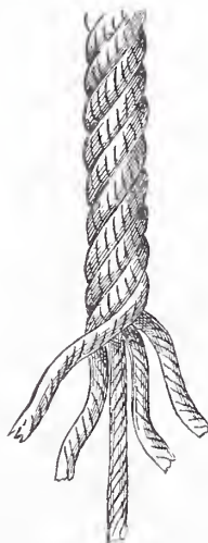
Fig. 2.—A "Shroud" Laid Rope. Four Strands, with a Core or Heart.
