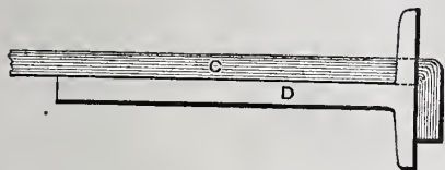
Anchors for Building.—Fig. 1.—Section showing Shape of Wrought Iron Strap.
