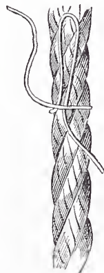
Fig. 5.—Manner of Laying the Twine in Commencing to Whip or Serve the End of a Rope.
