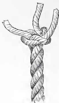
Fig. 21.—Side View of a Wall Knot after the Strands have been Drawn Tight.
