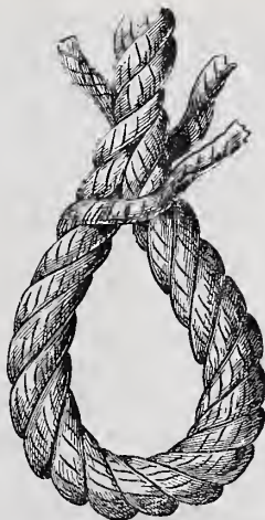
Fig. 44.—The Eye Turned, showing Disposition of Third Strand.
