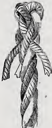
Fig. 17.—The Strands Drawn Tight, but not Fastened.
