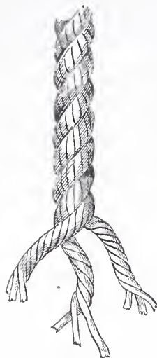
Fig. 1.—The Twisting of a Right Handed Rope.
