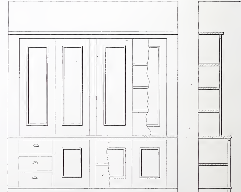
Fig. 39.—Elevation and Section of Pantry Shelving.—Scale, 3/8 Inch to the Foot.
