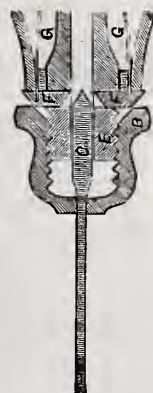
Fig. 5.—Showing the Clamp Removed, so as to Let the Tool Drop Into Reservoir.
