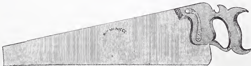
Fig. 2.—New Device for Fastening Saw Handles.—The Article Applied to a Panel Saw.
