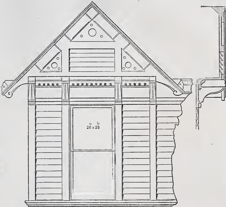
Fig. 14.—Elevation of Small Gable on North Side, with Second Story Window.—Scale, \frac{3}{8} Inch to the Foot.
