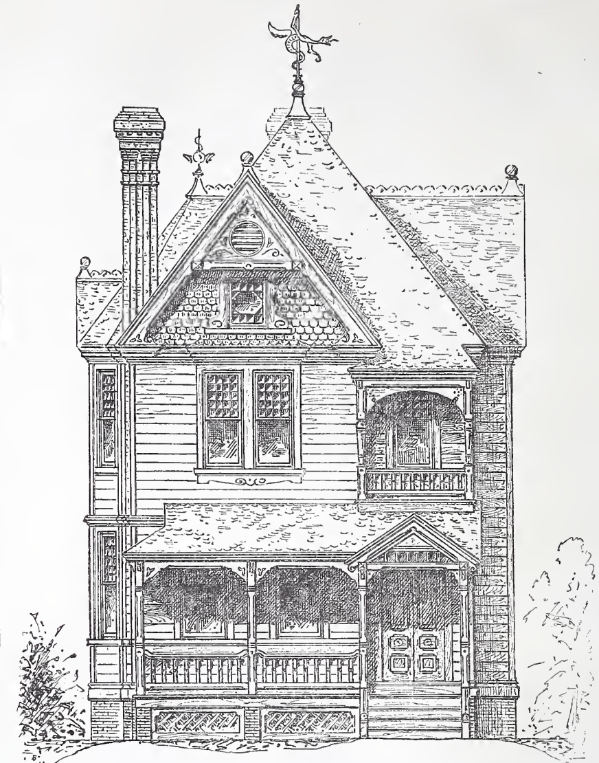
Fig. 4.—Front Elevation.—Scale, 1/8 Inch to the Foot.
