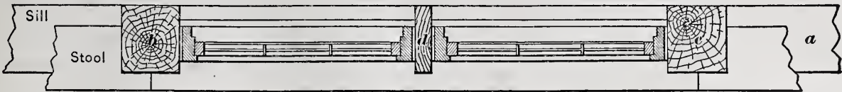
Fig. 4.—Horizontal Section, Main Window.—Scale, 1/2 Inch to the Foot.
