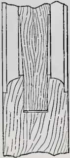
Fig. 13.—Section of Inside Doors.— Half-Full Size.
