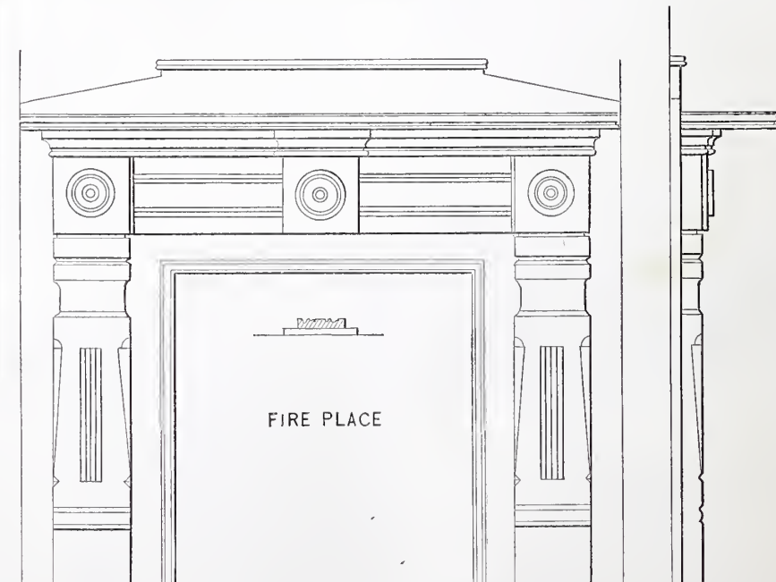
Fig. 28.—Elevation and Section of Sitting and Dining Room Mantels.—Scale, \frac{3}{4} Inch to the Foot.
