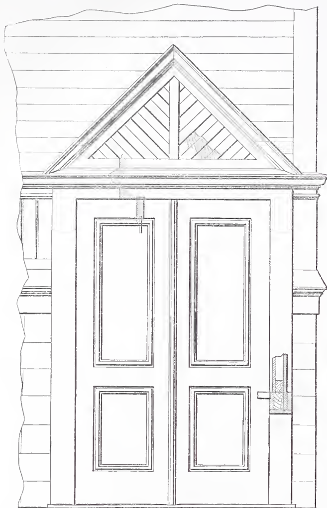
Study in Suburban Architecture.—Elevation of Entrance to Cellar.—Scale, \frac{1}{2} Inch to the Foot.
