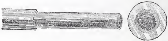
Fig. 4.—Full-Size View of End of Spindle and Section Through Socket in Knob.
