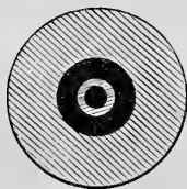
Fig. 4.—Cross-Section, Showing Pine Log Casing, Space and Steam Pipe.
