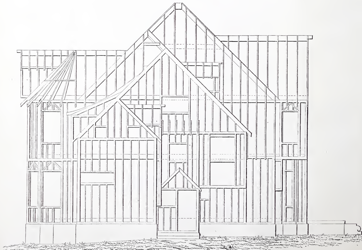
Framing Plan of North End.—Scale, \frac{1}{8} Inch to the Foot
