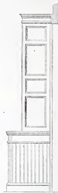
End Elevation of Dresser.—Scale, \frac{3}{8} Inch to the Foot.
