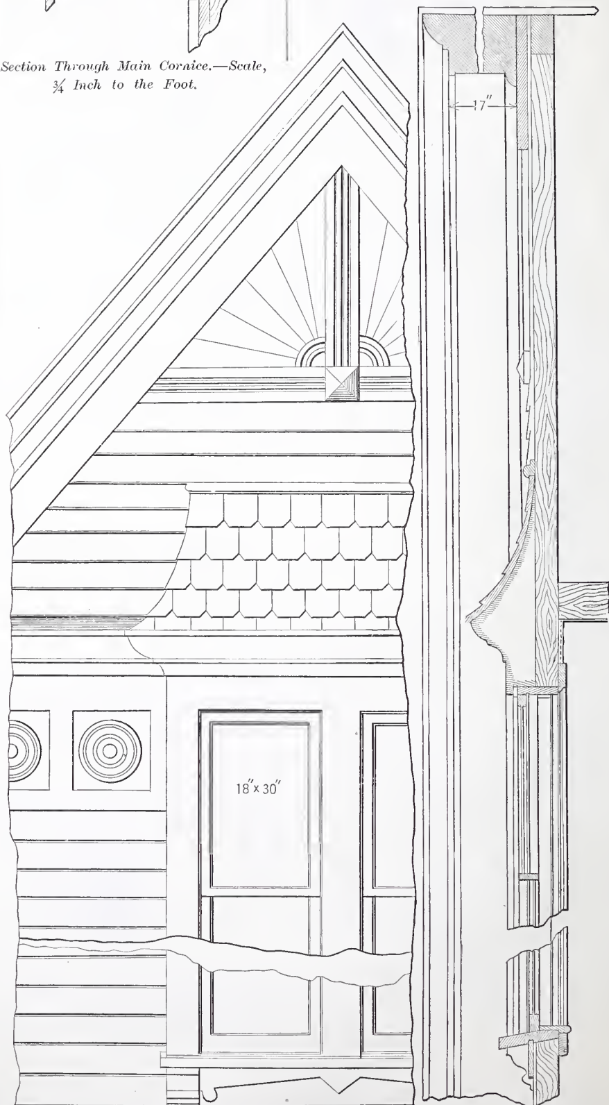
Details of Front Gable.—Scale, 1/2 Inch to the Foot.
