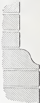
Base Course or Water Table of Molded Brick.
