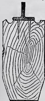
Fig. 7.—Section Through Bar of "Simplex-Laid" Glazing Before the Glass is Applied.
