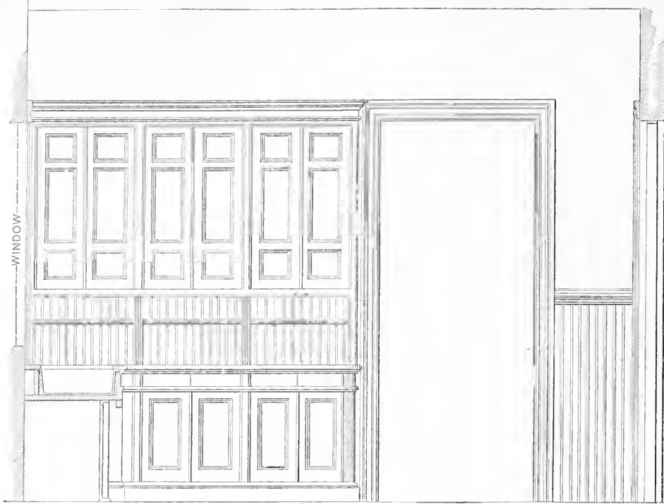
A Study in Suburban Architecture.—The Kitchen Finish.—Elevation of End of Kitchen, Looking Toward Dining-Room.—Scale, \frac{3}{8} Inch to the Foot.
