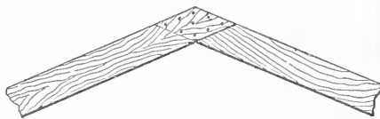
Fig. 3.—The Rafters are Halved Together, Primed and Nailed.—Dean's Patent.
