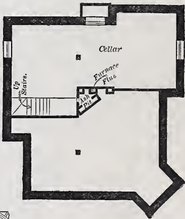
Cellar Plan.—Scale, \frac{1}{16} Inch to the Foot.
