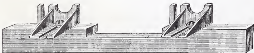
Fig. 2.—Filletster and Grooving Attachment, Having Reversible and Adjustable Wood Planer.
