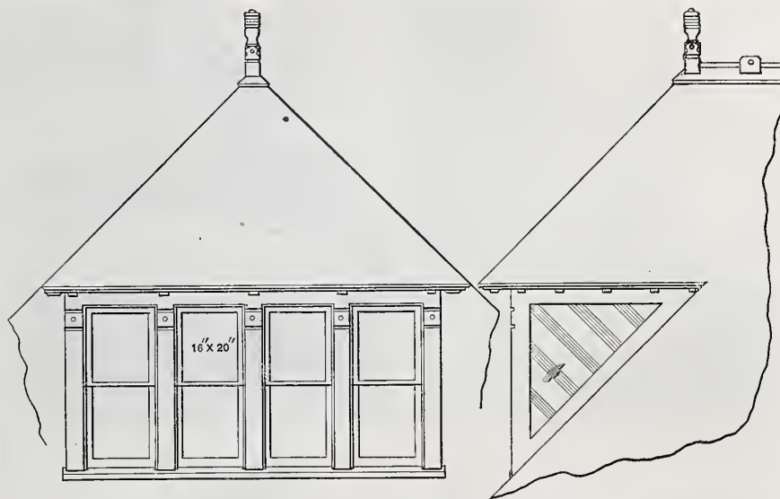
Figs. 15 and 16.—Front and Side Elevation of Rear Dormer in Wing.—Scale, \frac{1}{4} Inch to the Foot.
