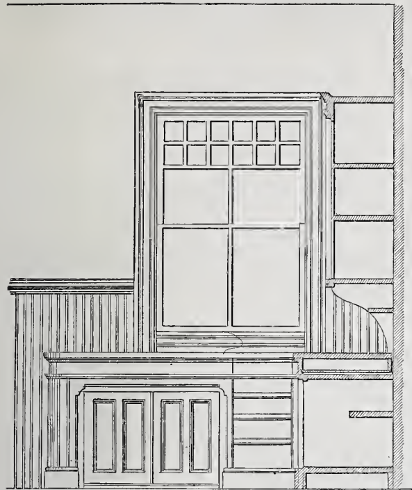
A Study in Suburban Architecture.—Elevation of Side of Kitchen, Showing Sink.—Scale, 3/8 Inch to the Foot.
