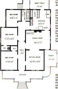
Floor Plan.-Scale, 1-16 Inch to the Foot.
