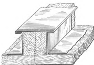
Fig. 14.—Edge of Cap Turned Over for Seaming.
