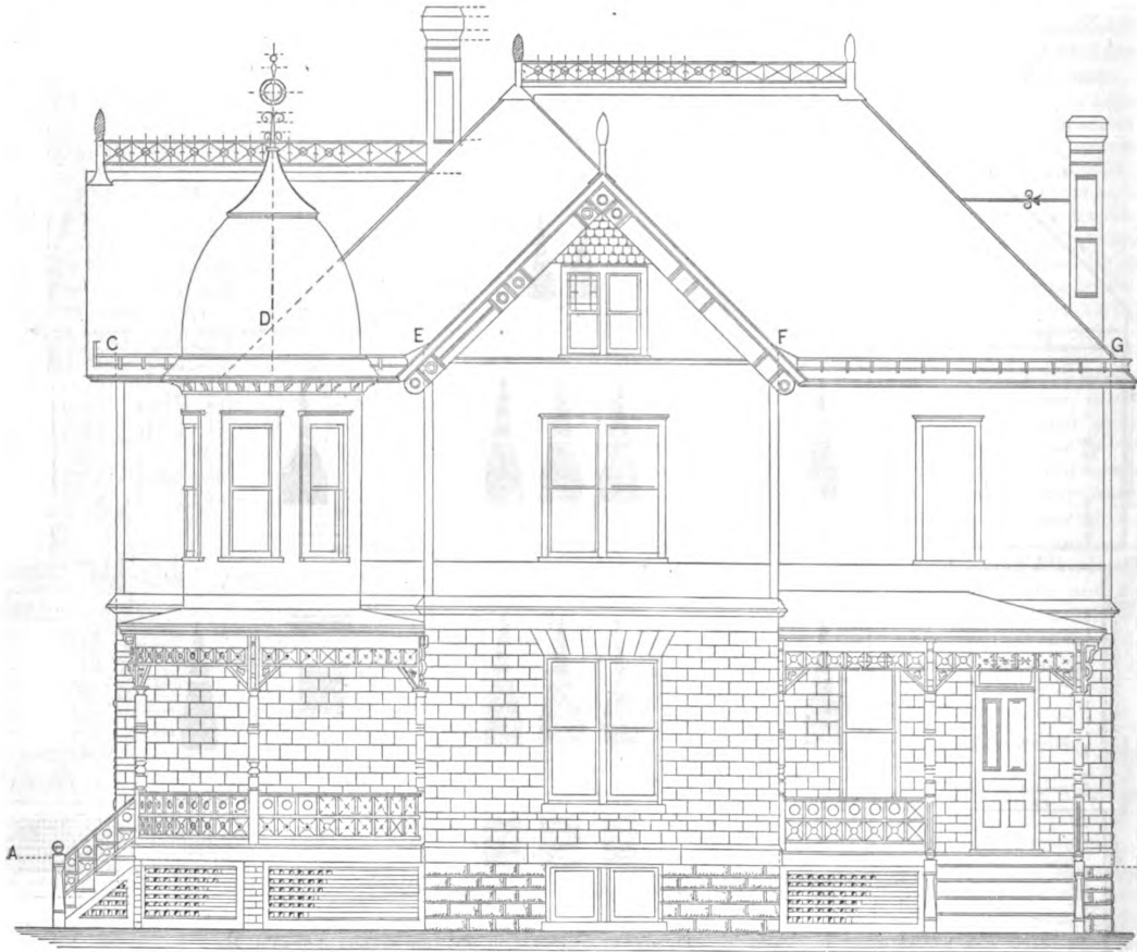
Architectural Drawing for Mechanics.—Fig. 39.—Side (Right) Elevation, showing Parts of the Work in Different Stages of Completion. —Scale, \frac{1}{4} Inch to the Foot.
