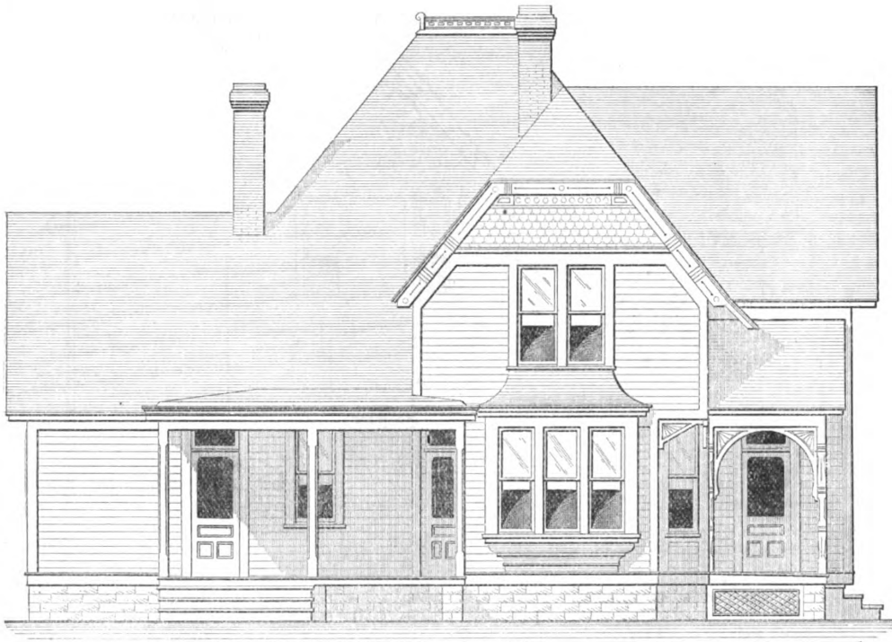
Design of a Suburban Cottage.—Side (Left) Elevation.—Scale, \frac{1}{8} Inch to the Foot.
