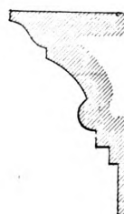
Detail of Counter Molding at B.—Scale, 3 Inches to the Foot.
