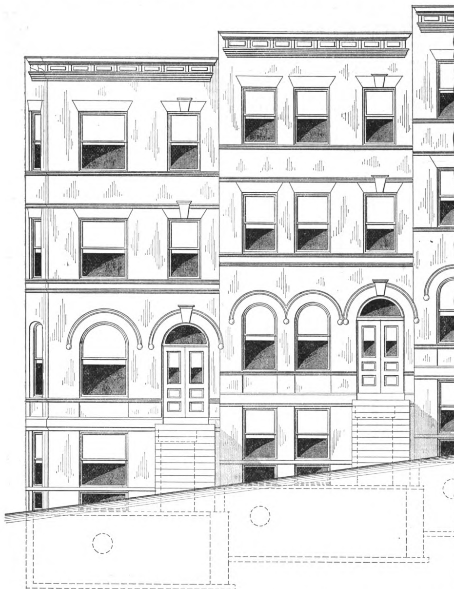
Front Elevations of the Two Houses shown at the Extreme Left on the Supplemental Plate.—Scale, \frac{1}{4} Inch to the Foot.
