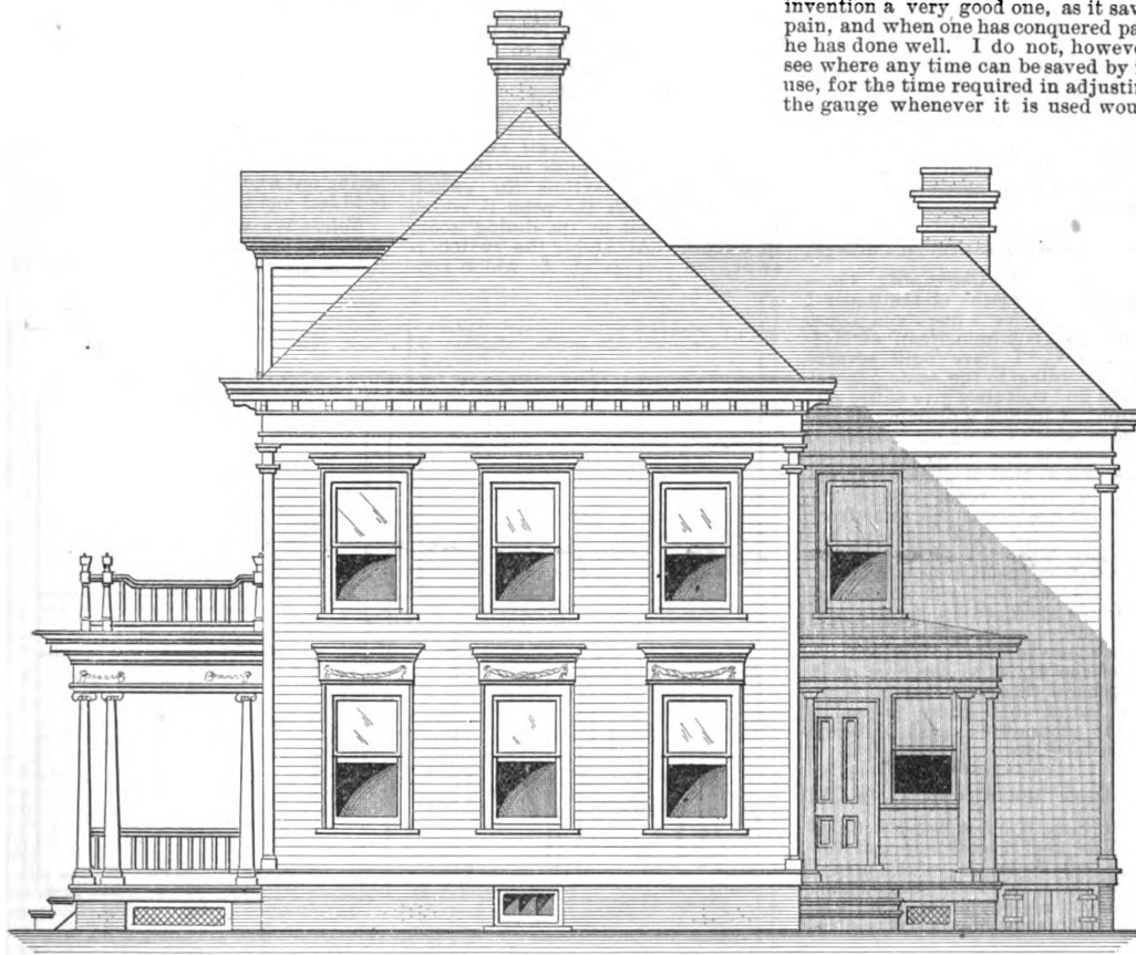
Side (Right) Elevation.—Scale, 1/8 Inch to the Foot.
