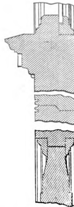
Section of Vestibule Door taken on Line A B.—Scale, 3 Inches to the Foot.
