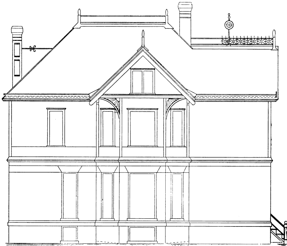
Architectural Drawing for Mechanics.—Fig. 40.—Side (Left) Elevation in General Outline.—Scale, \frac{1}{8} Inch to the Foot.
