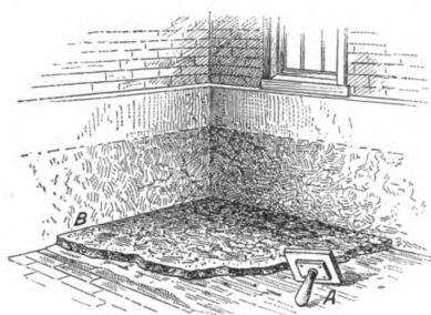
Fig. 5.—Applying the Coating of Mortar, Cement and Broken Stone to the Brick Work.
