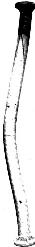
Fig. 4.—Cast Iron Column.—Load 84.8 tons, Temp. 1550°.
