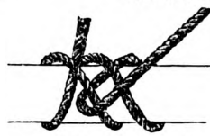
Fig. 20.—A Roll Hitch.
