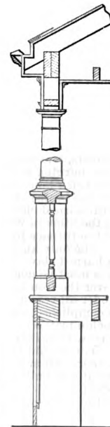
Details of Veranda Cornice, Columns, Balustrade, &c.—Scale, \frac{3}{4} Inch to the Foot.
