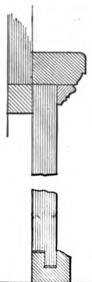
Fig. 15.—Detail of Wainscoting in Kitchen and Bathroom.—Scale, 3 Inches to the Foot.
