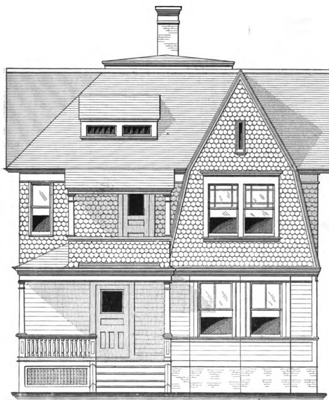
Front Elevation.—Scale, \frac{1}{4} Inch to the Foot.
