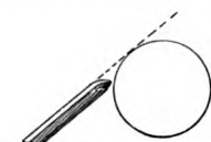
Fig. 23.—Angle for Starting Work with a Gouge.
