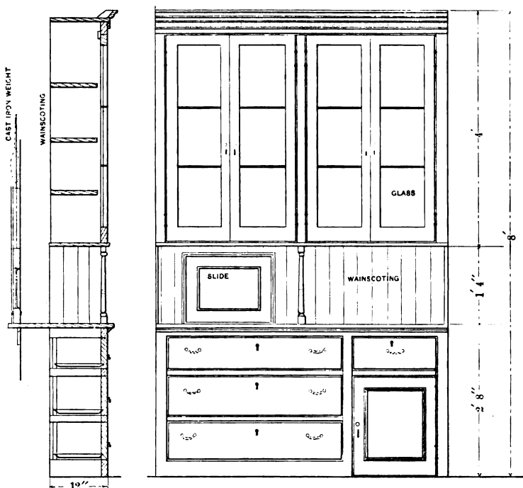
Vertical Section and Front Elevation of Case in Butler's Pantry—Scale, \frac{1}{4} Inch to the Foot.
