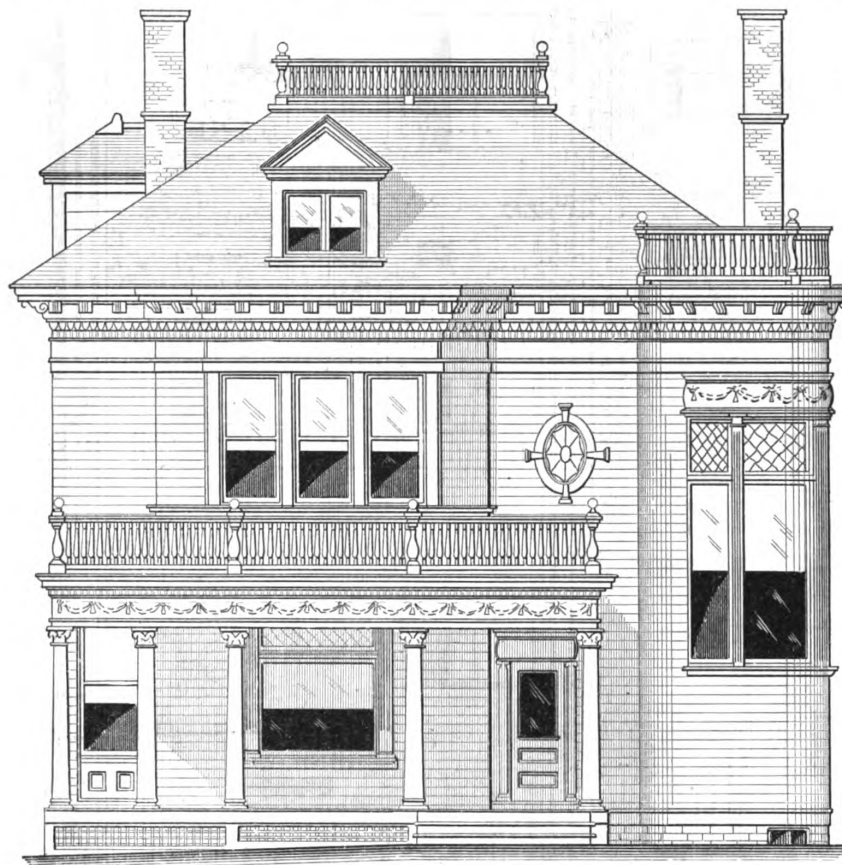
Front Elevation.—Scale, 1-8 Inch to the Foot.
