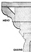
Detail of Door and Window Finish.—Scale, 3 Inches to the Foot.
