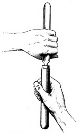
Fig. 22.—Manner of Holding a Gouge.
