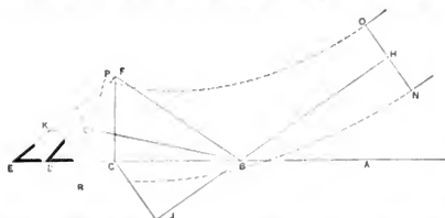
Method of Obtaining the Lines for Wreath Pieces in a Flight of Stairs the Plan of which is Less than a Quarter Circle.
