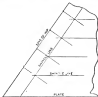
Fig. 2.—True Face of Roof, Showing Shingling Lines
