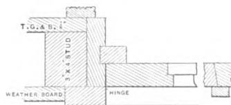
Horizontal Section through Door Frame. Scale, 1\frac{1}{2} Inches to the Foot.
