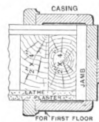
Section through Door Frame.—Scale, 1\frac{1}{2} Inches to the Foot.
