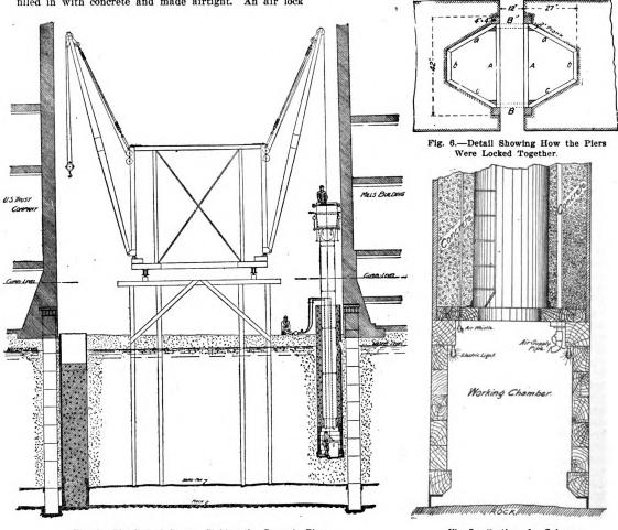
Fig. 4.-The Second Stage.-Sinking the Concrete Piers.
