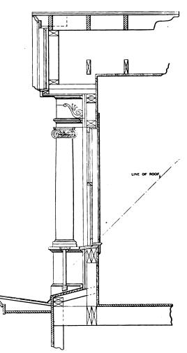
Section through Front Dormer .- Scale, 1/2 In. to the Foot.
