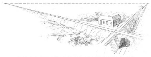
Fig. 2.-Finding Vanishing Points by Observation on Two Railroads Crossing Each Other.
