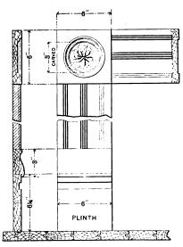
Details of Door and Window Trim .- Scale, % In. to the Foot.
