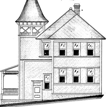
Design for Four-Room Schoolhouse .-- Side (Right) Elevation .-- Scale, 1/8 In. to the Foot.
