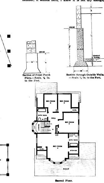
Hollow Concrete Block Residence at Bay Bridge, Ohio.-Floor Plans.-Scale. 1-16 In. to the Foot.
