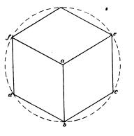
Fig. 1.--Isometrical Projection of a Cube.
