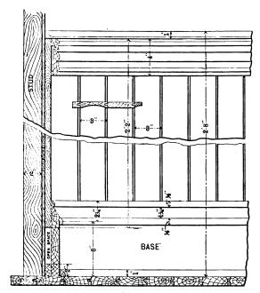
Details of Wainscoting, Base and Cap Molding in Kitchens and Bathrooms.—Scale, 1½ In. to the Foot.
