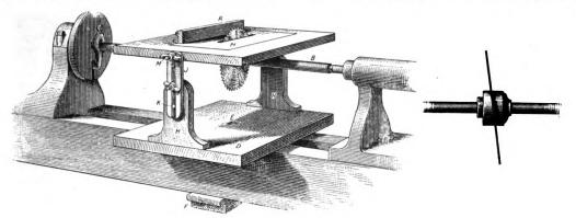
Fig. 2.-Circular Saw Attachment for Lathe.
