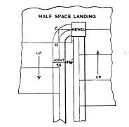
Fig. 2.—Partial Plan Showing Method Where a Small Curve Is Placed at Bottom of Return Flight.
