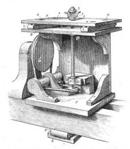
Fig. 1.-Molding Machine Attachment for Wood Turning Lathe.
