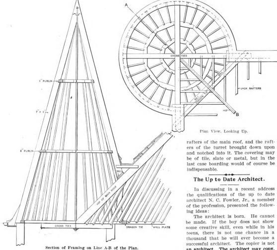
Framing a Conical Roof.
