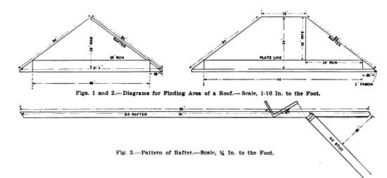
Estimating Roof Construction.-Diagrams Submitted by S. E. J.
