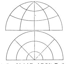
Constructing a Spherical Shaped Skylight—Elevation and Plan.
