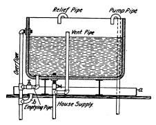
Pipe Connections at a House Tank.
