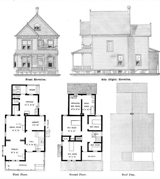
Elevations for "A. E. P.'s" Floor Plans.
