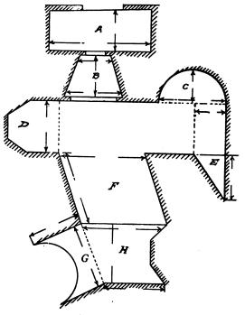
Diagram Showing Correct Method of Measuring Floors and Walls for Tiling.
