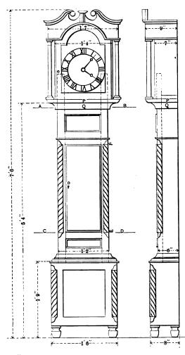
Front and Side Elevations .- Scale, % In. to the Foot.
