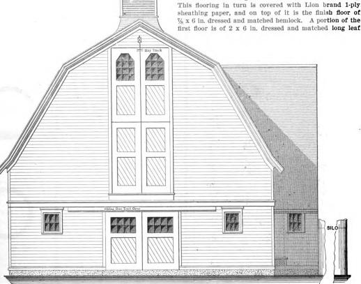
made by the Stowell Mfg. & Foundry Company, Chicago, and run on steel track. The doors are supplied with wall stay rollers, upper and lower front binders and pulls.
