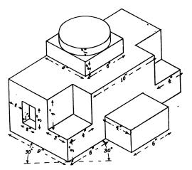
Fig. 2.—Isometrical Drawing of an Object Shewing Method of Scaling the Measurements.
