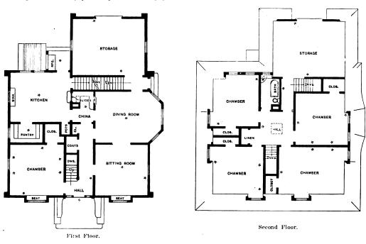
Design of a Gardener's Cottage-Floor Plan-Scale, 1-16 In. to the Foot.
