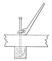
Handy Method of Withdrawing a Bolt.
