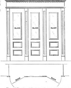
Plan and Elevation of Wardrobe.-Scale, % In. to the Foot.
