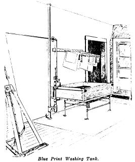
best service of any of the schemes the writer has tried. A standing waste as purchased has the overflow too high, but it is only necessary to drill some holes in the stand pipe at the proper level, after the waste is in place.
