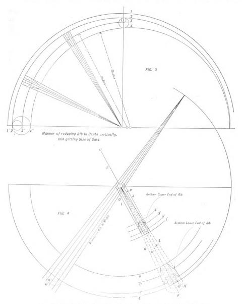
Figs. 3 and 4.-Method of Reducing the Ribs and Obtaining the Sections Thereof.
