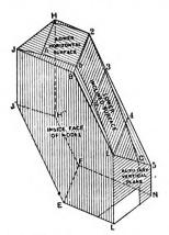
Fig. 65.-Oblique Projection of Model of Fig. 64, Also Showing Application of Patterns to Low Surfaces of Plank, Figs. 54 to 58.
