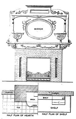
Plans and Elevations of Mantel in Parlors.-Scale, % In. to the Foot.
