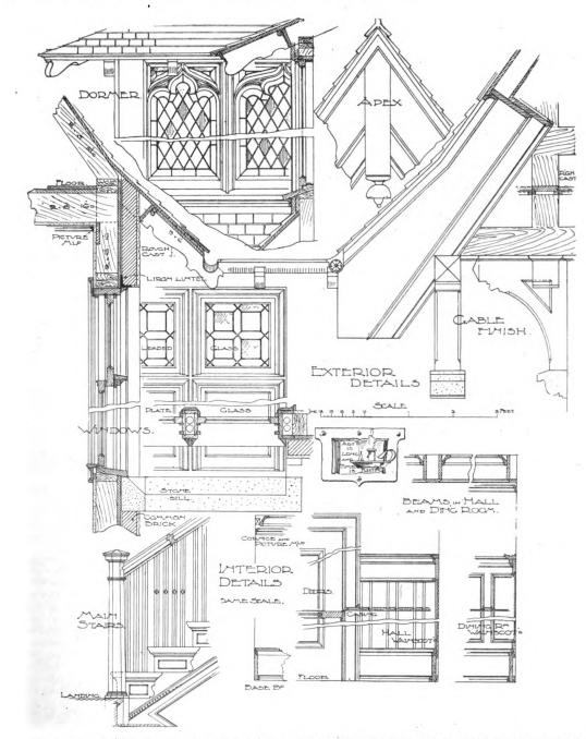
Competition in \$8000 Houses .- First Prize Design .- Reduced Facsimile of Sheet of Architect's Drawings Showing Miscellaneous Constructive Details.
