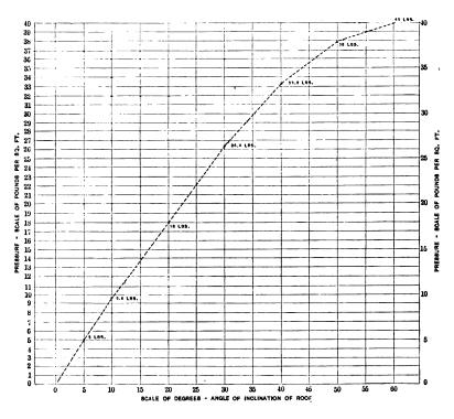
Diagram Illustrating Formulæ for Figuring Wind Pressure on a Roof.
