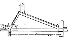
Fig. 4.—Saw-Tooth Skylight in Reinforced Concrete, with Heavy Concrete Beam as the Bottom Chord of the Truss.
