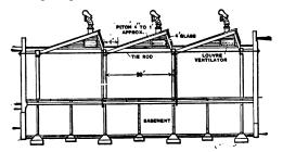
Fig. 1.—Standard Saw Tooth Skylight in Mill Construction.— Fiberioid Company's Plant at Indian Orchard, Mass—Flat Roof Between Skylight and Ventilators.
