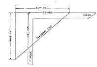
Finding the Rise of Roof Per Foot Run-Diagram Accompanying Letter of "D. L. C."
