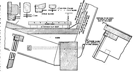
Fig. 2.-Detail of Americanized Saw-Tooth Skylight for Factory Roofs.
