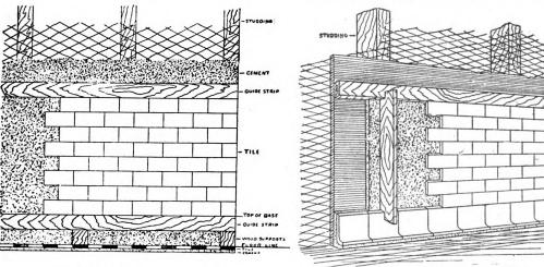
Fig. 7.-Method of Laying Wall Tile.
