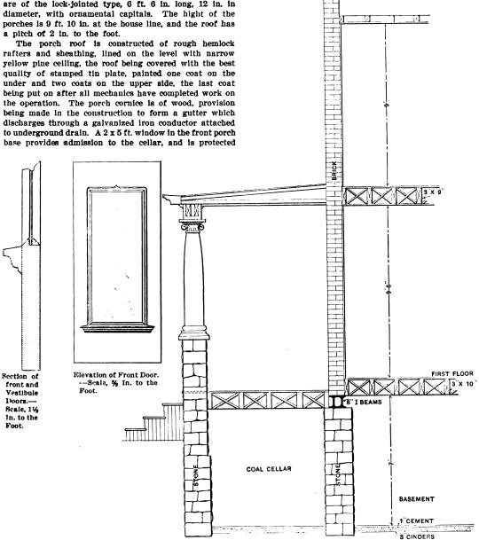
Section through Front Wall and Porch .- Scale, ¼ In. to the Foot.
