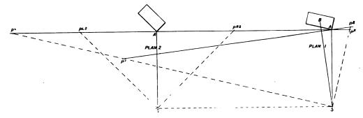
Fig. 6.--Comparison of Distance to Vanishing Points in Different Angles of View.
