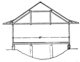
Fig. 1 .-- Cross Section of Freight Shed .-- Scale, 1-16 In. to the Foot.
