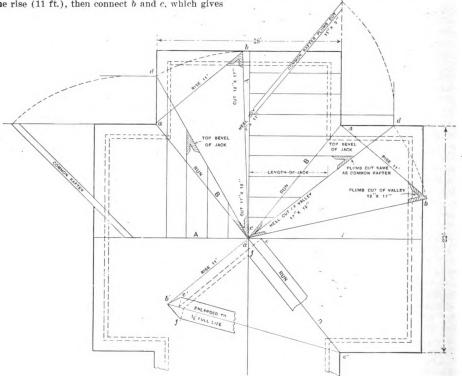
Finding Side Cut of Valley Rafter in Roof of Unequal Pitch.
