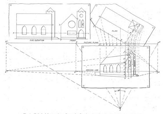
Fig. 4.-Method of Constructing a Perspective Drawing According to the "Plan Above" System.
