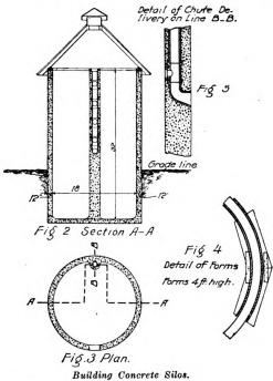
lengths of plain pipe and tees are used, so as to bring the openings 4 ft. apart, as indicated in Fig. 5. Terra cotta plugs are used when filling and these are removed as the silo is emptied, thus giving access to the chute from the inside.
