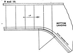
Fig. 13.—Plan of Stairway Having a Curve Less Than a Quadrant at the Bottom, the Wreath Connecting Both the Level Rail and the Rail of the Flight Adjoining. PLAN PLAN
