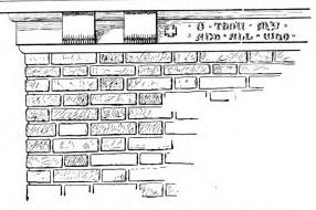
Partial Elevation of Chimney Breast in Living Room.--Scale, ¾ In. to the Foot.
