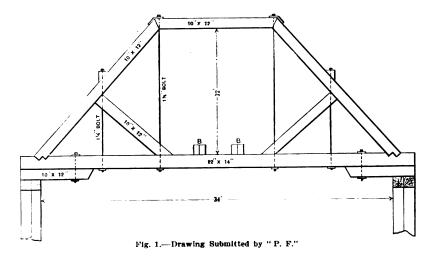
Finding Safe Load for Truss of 34-Ft. Span.
