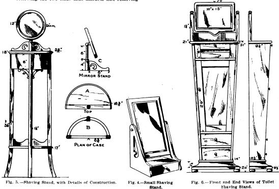
Cabinet Work for the Carpenter.-The Bathroom.
