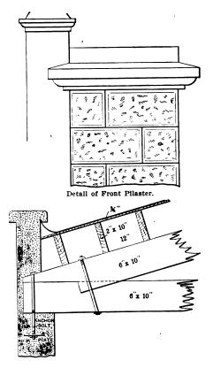
Detail of Roof Truss .- Scale, 1/2 In. to the Foot.
