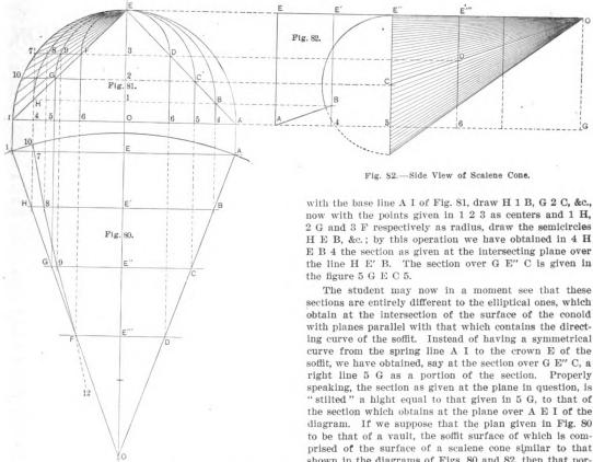
Figs. 80 and 81 .- Plan and Elevation of Scalene Cone, with Developed Sections at the Planes H E B, &c., of Fig. 80.
