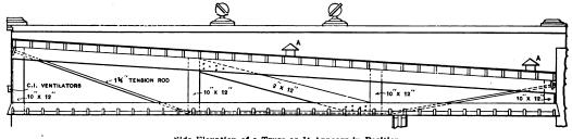
Side Elevation of a Truss as It Appears in Position.
