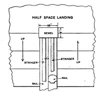
Fig. 1.—Part Plan Showing How to Treat the First Two Flights Connecting with the First Landing Newel.
