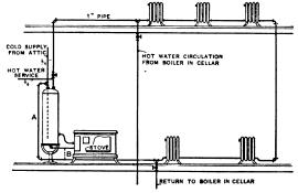
Fig. 2.—The Proposed Heating System.
