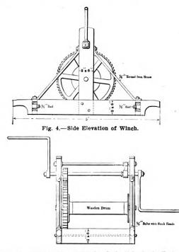
Fig. 5.-End Elevation of Winch.-Scale, 1/2 In. to the Foot.
