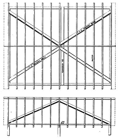
Trussing Roofs to Prevent Spreading and Sagging.
