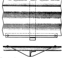
Fastening Corrugated Roofing Sheets to Rafters.
