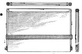
Fig. 1.—General View of Upright Drawing Table, with Movable Fig. 2.—Drawing Board, with Movable Straight Edge Operated by Means of Cords and Pulleys.
