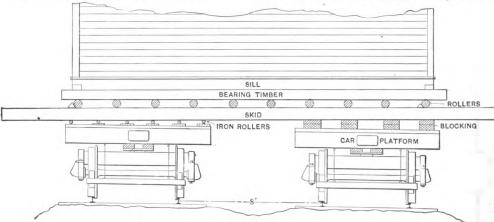
Fig. 3.-End Elevation of Building, Showing Skids, Cars, &c.
