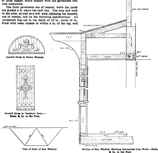
Miscellaneous Constructive Details of a Typical Philadelphia Building Operation.
