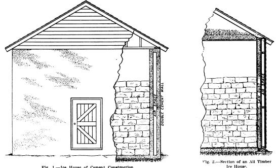
Fig. 1 .--- Ice House of Cement Construction.
