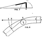
Fig. 7.-Bevel to the Wreath Shown in Fig. 8. Fig. 8.-Face Mold for the Wreath Shown in Figs. 5 and 6.
