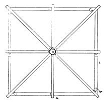
Fig. 4.--Plan of Louver Showing Structural Iron Framing.
