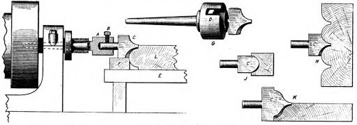
Fig. 3.-Molding Arrangement for Lathe and Method of Overcoming Danger of Exposed Bolt Heads.
