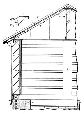
Fig. 9 .-- Vertical Section, Showing Sheet Metal Work
