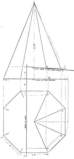
Fig. 1.-Plan and Elevation of Tower Framing.
