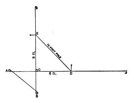
Fig. 5.-Squaring the Corner by Means of Tape Line or Pole.
