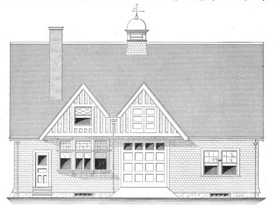
Front Elevation .- Scale, 1/8 In. to the Foot.
