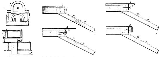
Figs. 5 and 6.—" Drip " for Patent Roll Cap.
