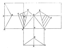
Finding Side Cut of Valley Rafter in Roof of Unequal Pitch.
