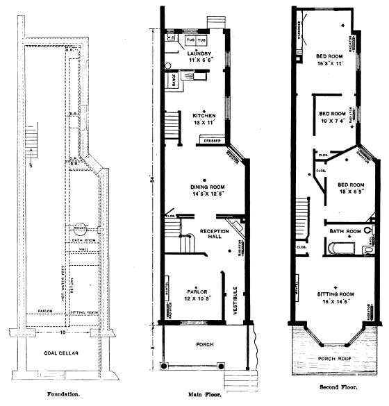
A Typical Philadelphia Building Operation.—Floor Plans.—Scale 1-16 In. to the Fout.
