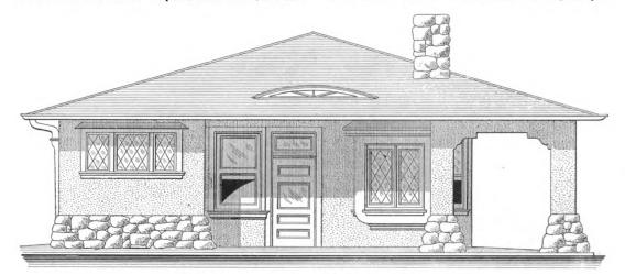
Street Elevation of Station .- Scale, 1/8 In. to the Foot.
