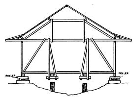
Fig. 2.—Showing How Braces and Hangers Were Applied.— Scale, 1-16 In. to the Foot.
