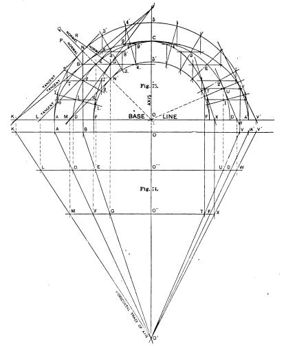
Figs. 74 and 75 .- Problem in Geometry Relating to Generation of a Right Conold.
