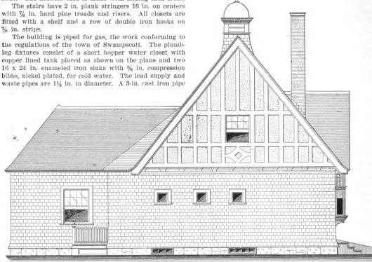
Side (Left) Elevation .- Scale, 1/8 In. to the Foot.
