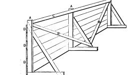
Fig. 9.—Treatment of Joist Spaces to Exclude Cold and Vermin.
