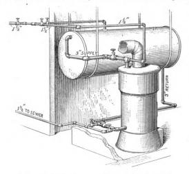
Fig. 3 -Heating Apparatus for the Swimming Pool.
