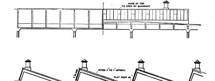
Fig. 5.-Saw-Tooth Skylight in Reinforced Concrete, with the Bottom Chord of Trussed Form Simply a Tie Rod at the Column Line.
