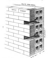
Detail of Brick Veneered Hollow Block Terra Cotta Wall.
