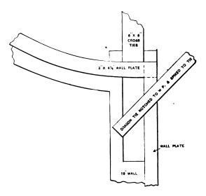
Detail Showing Construction at the Angles.
