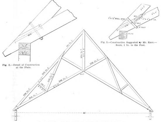
Fig. 1.-Elevation of Truss, with Stresses in the Several Members Shown.
