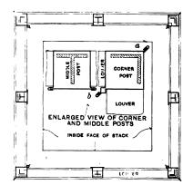
Figs. 6 and 7.—Showing Manner of Connecting the Base of Louver to Brickwork.
