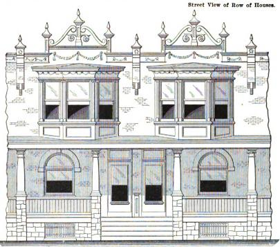
Front Elevation of Two of the Houses .- Scale, 1/4 In. to the Foot.
