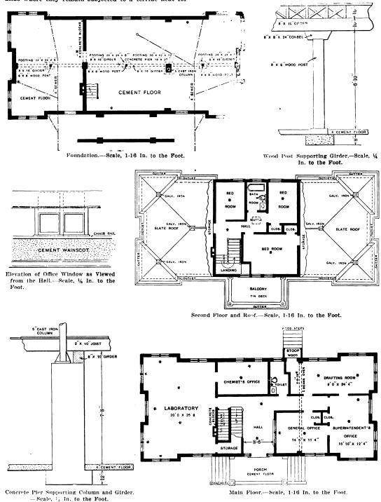
Concrete Block Office Building .- Floor Plans and Miscellaneous Constructive Details.
