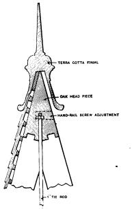
Detail at Apex of Roof.
