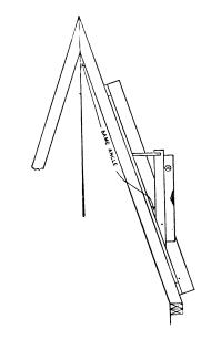
Fig. 2.-Method Employed for "Plumbing" the Tower Roof with Level and Straight Edge.
