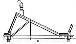
Fig. 3.-Elaborate Trussed Form of Saw-Tooth Skylight.
