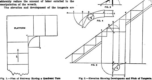
Fig. 1.—Plan of Stairway Having a Quadrant Turn Between Two Flights Placed at Right Angles to Each Other.
