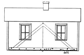
Fig. 3.—Side Elevation of Building, Showing How 6 x 9's Were Applied.—Dotted Lines Show Proposed Truss, Which Was Not Neccessary.—Scale, 1% In. to the Foot.
