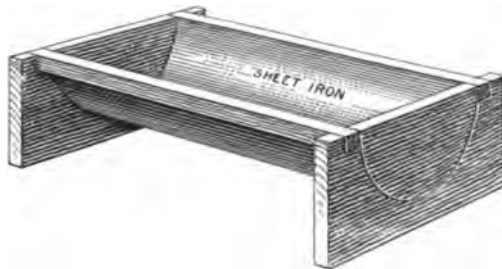
Fig. 93.—Alternate Method of Making Core Box.
