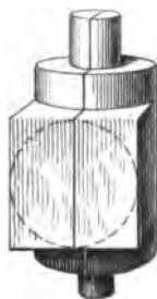
Fig. 72. — Joint in Block Corresponds with Joint in Valve Seat.
