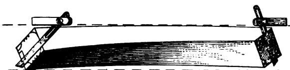
Fig. 28.—Showing the Appearance of Wreath for the Stretchout Curve After It Is Squared and the Bevels Applied.
