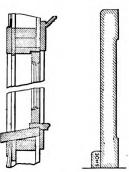
Detail of Casement Window.—Scale, % In. to the Foot.
