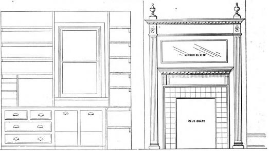
Details of Pantry Finish .- Scale, % In. to the Foot.
