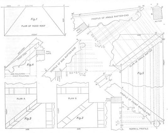
Rafter-End Under Hip Between Roofs of Unequal Pitch .- Diagrams Showing How to Do the Work.
