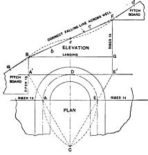
Fig. 3.—Method of Finding Correct Angle of Falling Line of Rail-Across Well Hole.
