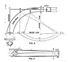
Fig. 3.—Method of Laying Out Face Mold by Means of String and Pins.
