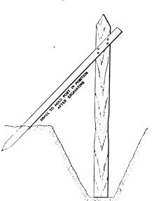
Fig. 1.-Post Braced in Position
