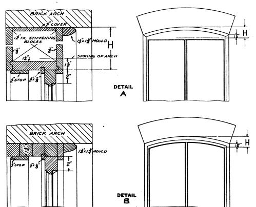
Figuring the Hight of the Springing for Circular Headed Window Sash.
