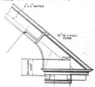
Detail of Main Cornice for Last Two Houses in the Row.— Scale, % In. to the Foot.
