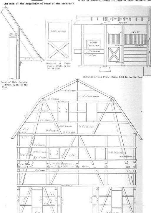
West End Elevation, Showing Framing .- Scale, 1/2 In. to the Foot.
