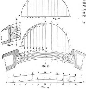
Fig. 21.-Plan of Window Frame in Circular Wall.
