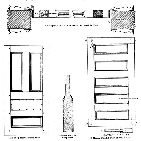
Making a Metal Covered Door.—Miscellaneous Details, Showing Construction.
