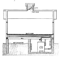
Fig. 1.—Vertical Cross Section of Kiln, Showing General Arrangement.
