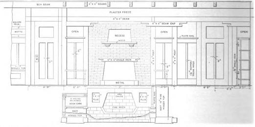
Elevation and Plan of Fireplace with View in Living Room Looking Toward the West, or Rear, and Showing Hall Door to the Left and Dining Nook to the Right.—Scale, ¼ In. to the Foot.
