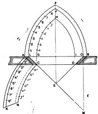
Fig. 26.—An Opening in a Straight Wall with Splayed Jambs and Pointed Soffit.
