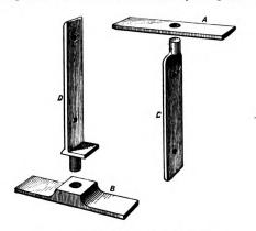
Fig. 3.—Details of the Upper and Lower Shoes,
