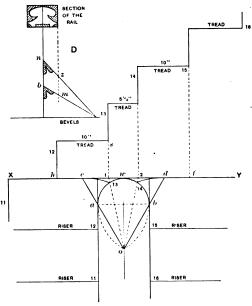
Determining Lengths of Treads in Stair Construction.
