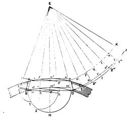
Fig. 28.—An Opening in a Circular Wall with Jambs and Circular Heads Splayed Equally.
