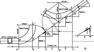
Fig. 74.—Showing Elevation of Steps, Pitch Line of Tangents and Face Molds
