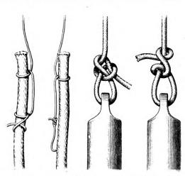
Figs. 62 and 63.—Methods of Attaching "Mouse" to Cord.
