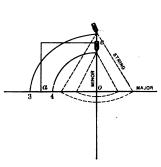
Fig. 75.—Face Mold for Bottom Wreath, the Curves Being Drawn by Means of Pins and String.
