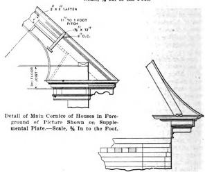
Detail of Tower Cornice of Last House in the Row.—Scale, % In. to the Foot.
