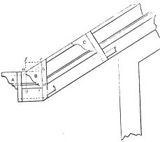
Cutting Raking Moldings as Suggested by "C. J. M."
