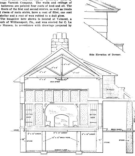
Cross Section of Building, Showing Roof Construction .- Scale, 44 In. to the Foot
