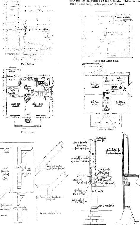
Developing the Plans for a Workingman's Home.—Scale of Floor Plans 1-16 In. to the Foot.
