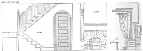
Section and Elevation of Main Staircase. Elevation of Hall Mantel. "Nook," Looking Toward the Hall.
