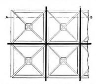
Fig. 2.—Plan of a Floor Slab, the Heavy Black Lines Indicating the Reinforcing Rods Running at Right Angles to Each Other.
