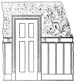
Elevation of Dining Room Wainscoting and Plate Rail, Showing Pantry Door .- Scale, % In. to the Foot.
