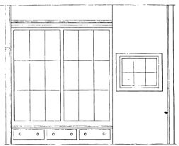
Elevation of Harness Closet .- Scale, 1/4 In. to the Foot.
