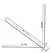
Fig. 1.—Plan of Corner of Building, Showing Seat of Hip Rafter. Fig. 2.—Showing Method Where the Hip Rafter Is Concave in
