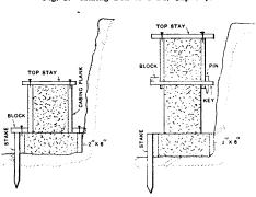
Fig. 3 .-- Section Showing Footing and First Layer of Wall.
