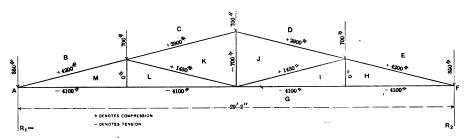
Truss Diagram .- Scale, 3-16 In. to the Foot.
