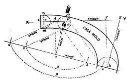
Fig. 61 .- Face Mold for the Wreath Shown in Fig. 60.
