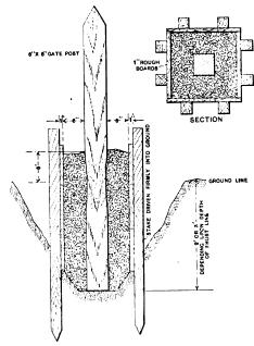
Fig. 2.—Details of the Concrete Work.
