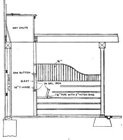
Vertical Longitudinal Section Through Stalls.—Scale, 3-16 In. to the Foot.
