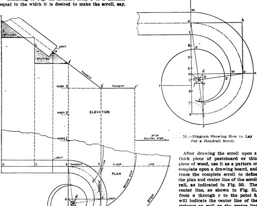
Fig. 50 .- Plan of Scroll and Sweep Steps; Also Elevation of the Plan Scroll Tangents 4-b and b-c.
