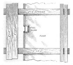
A Simple Scaffold for Iron Workers' Use.—Fig. 1.—Plan View, Showing General Arrangement of Parts.
