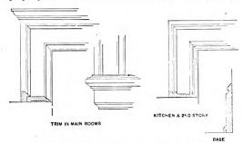
Details of Interior Finish.—Scale, 1 In. to the Foot.
