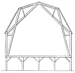
Inside Bent of Plank Frame Barn, Showing Construction for Which Truss Diagram Is Wanted,
