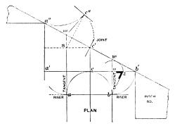
Fig. 1.—Plan and Elevation of Tangents for a Wreath Over a Half-Space Platform Cylinder.
