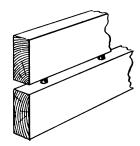
Fig. 20.-A Doweled Joint,
