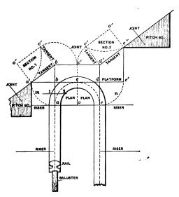
Fig. 39.—Plan and Elevation of Tangents for a Half Space Landing Stairway.
