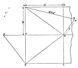
Fig. 1.—Plan of Hip Roof.
