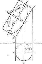
Fig. 49.—Drawing an Ellipse with String and Pins.
