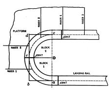
Fig. 72.--Plan of Cylinder and Steps Adjoining.
