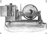
Fig. 11.—The Polygon Concrete Mixer.
