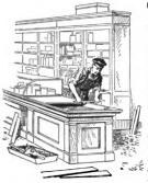
HE method of cleaning off our counter top will depend somewhat upon the size of it. Wherever possible it is generally better to straighten the bottom side and the edges and fasten it in place before trying to dress off the top. Where it is not possible to do this and the top shows a tendency to curl or warp two or three stout cleats may be temporarily fastened to the under side of it, but even then the final
