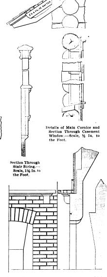
Partial Elevation and Section of Fireplace in Dining Room .- Scale, 1/2 In. to the Foot.
