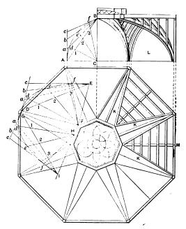
Fig. 18.—An Octagonal Apartment with a Groined Ceiling and an Octagonal Skylight.
