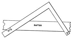
Fig. 3 .- Finding the Cut with the Steel Square.
