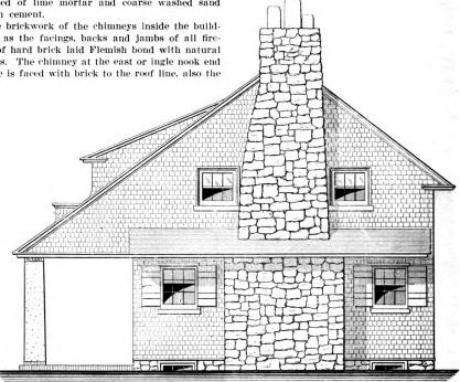
East End Elevation, Showing Chimney Construction.-Scale, 1/8 In. to the Foot.
