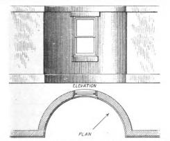
Fig. 3 .- Showing Method of Shading a Concave Wall Surface.
