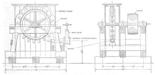
Side and End Elevations of a 3-Ft. Diameter Impulse Water Wheel.
