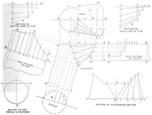
Fig. 2.- Design for Elbow and Method of Developing Patterns for It.
