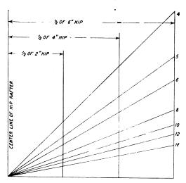
Fig. 2.—Diagram Showing Line of Bevel for Different Pitches.
