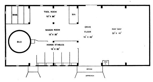
Main Floor, Showing Hay Bay, Horse Stalls, Tool Room, &c .- Floor Is of Reinforced Concrete.
