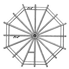
Fig. 1.—Plan of Roof for Silo Submitted by "G. A. W."
