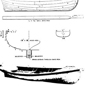
Building Sheet Metal Boats.—General View of Completed Boat and Parts of Which It Is Composed.
