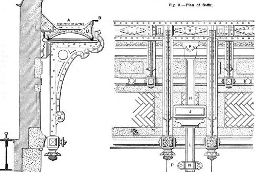
Fig. 1.—Section of Gutter and Leader.
