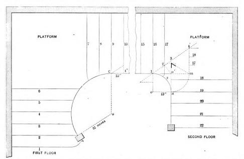
Fig. 65.—Plan of a Cylinder Stairway Containing Stretchout Curve More Than a Quadrant at the Starting, a Quarter Turn at the Intersection of the Two Flights and a Goose Neck Curve on the Rail Connecting the Newel of the Second Story Landing.
