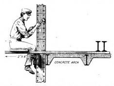
Fig. 2.—Side Elevation of Scaffold, Showing Workman Holding Hammer While Riveting Gun Is In Use.
