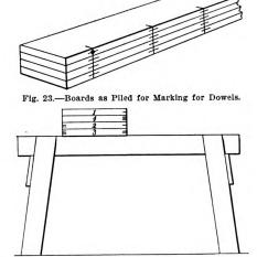
Fig. 22.—End View of Boards Arranged on Trestles Ready for Gluing.
