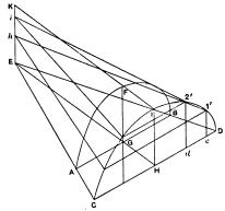
Fig. 30.—Isometrical Projection of Cone-Like Solid, the Surface of Which Corresponds to the Contour of the Inside of the
