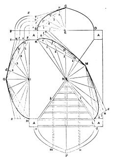
Fig. 4.—Curves Found by Intersecting Lines.
