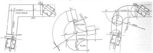
Fig. 81.—Face Mold for a Square Rail Around the Corners Shown in Plan, Fig. 77.
