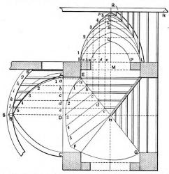
Fig. 11.—A Gothic Groined Vault with the Summit of the Side Arches Joined to the Summit of the Body Range by a Curved Ridge.
