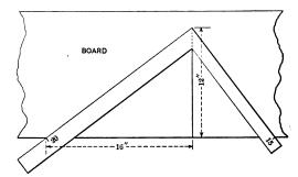
Fig. 2 .- Using the Steel Square in Solving the Problem.
