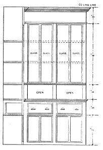
Section and Elevation of Pantry Cupboard .- Scale,
