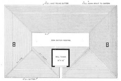
Plan of Roof .- Scale, 1-16 In. to the Foot.
