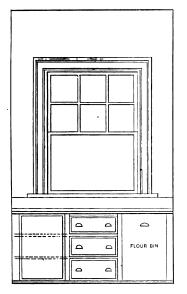
Elevation of Pantry Shelf .- Scale, % In. to the Foot.
