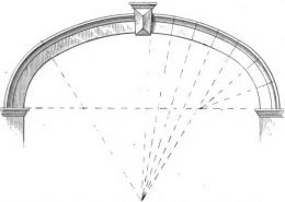
Fig. 4 .- A Semi-Elliptical Arch Described from Three Centers.
