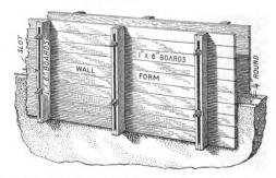
Perspective of a Section of Wall Showing Manner of Construction.
