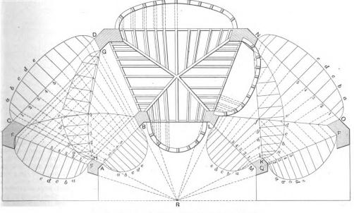
Fig. 12.—Diagrams Showing Groining on an Octagonal Plan.
