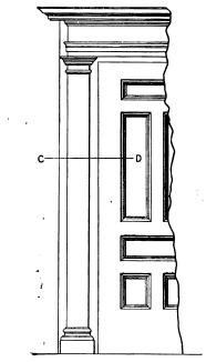
Fig. 3.—Partial Elevation Showing "Grounds" Under Pilaster Next to Plastered Wall.
