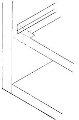
Fig. 51. Showing the Manner in Which the Shelf Is Fitted.--Scale, 3 In, to the Foot.
