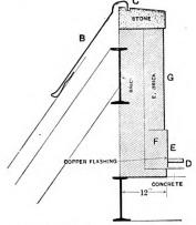
Fig. 3 .- Method of Making Water Tight Connection.
