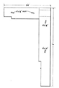
Fig. 1.-The Two Pieces of 2 x 8 In. Stock Mortised Together.
