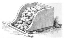
Fig. 3.—Showing Use of Running Rods in Keeping Parts of Mold Together.
