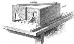
Fig. 2.—The Reverse Mold for Casting the Column.
