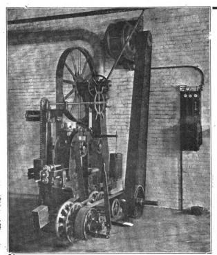
Fig. 502 American 48" Band Re-saw, with Motor, Belt Driven
