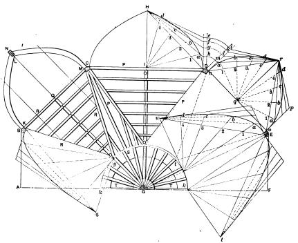
Fig. 19.—A Groined Vault on an Irregular Octagonal Plan.
