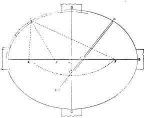
Fig. 3.—Showing Method of Making Templates for the Different Pieces of Curved Paneling.
