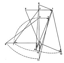
Fig. 2.—Diagram for Finding Lengths and Bevels.
