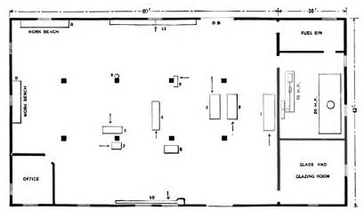
No. 1 is a 7-in. Sticker; 2 is a Single Planer; 3 is a Rip Saw; 4 is a Universal Woodworker; 5 is a Single-Spindle Shaper; 6 is a No. 2 Mortiser; 7 is a Band Saw; 8 is a Tenoning Machine; 9 is a Sandpapering Machine; 10 is a 16-in. Turning Lathe; 11 is a Swing Catalogue.
