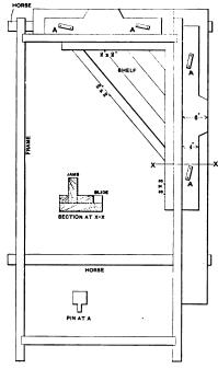
Fig. 2.—The Frame or Clamp Complete with Details of Construction.
