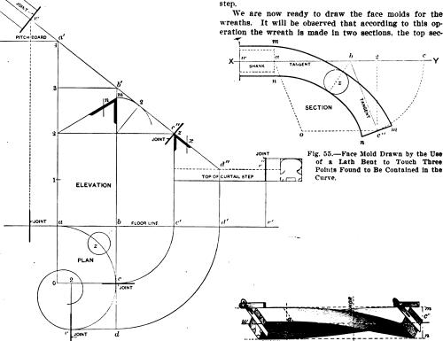
Fig. 54.-Plan and Elevation of Scroll Hand Rail Covering Two
