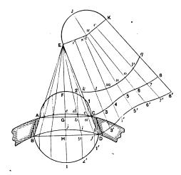
Fig. 31.-An Opening in a Circular Wall with Splayed Jambs and Circular Head Following Level at the Crown.
