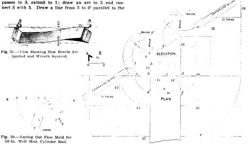
Fig. 29.-Plan, Elevation and Development of Tangents and Center Line of Rail for the 10-In. Cylinder of the Well Hole.
