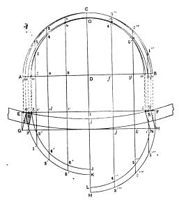
Fig. 37.—Development of Molds for Cote Bar.
