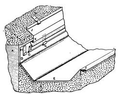
Fig. 4.—Construction of Copper Gutter.
