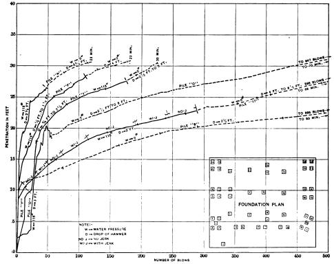
Fig. 6.-Diagram of Concrete Pile Curves, Showing Characteristics of Driving.
