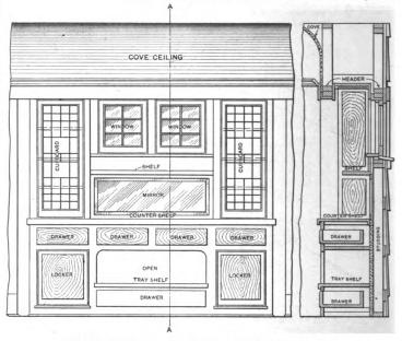
Elevation and Section at A-A of Breakfast Room Buffet.—Scale, % In. to the Foot.
