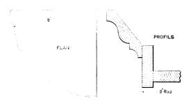
Setting Out a Splayed Crown Molding for Circular Cornicc.
