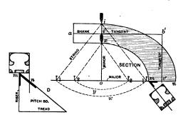
Fig. 52 .-- Face Mold for the Wreath Rail.
