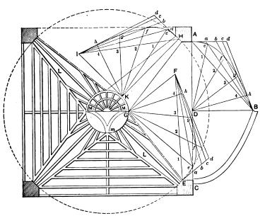
Fig. 15.—A Spheroidal Vault Intersected by Two Gothic Vaults at Right Angles and Having a "Drop" in the Center.
