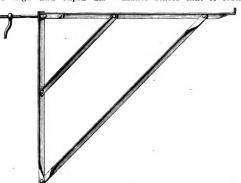
Novelties .- Fig. 4 .- A New Folding Steel Builder's Bracket.
