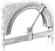
Fig. 1.—Method of Running a Semicircular
