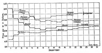
Fig. 2.—Totaled Average Costs of Brickwork on Four Buildings.
