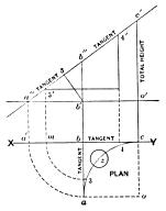
Fig. 44.—Diagram Showing Elevation of Tangents Over the Cylinder.
