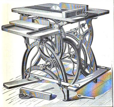
Iron frame 36 inches high. Center part of top is made of iron accu-rately planed with grooves on each side of saw for gauges to slide in. Steel shafts and best babbitt metal boxes.
