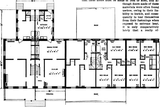
Floor Plans of House of Type No. 6 .- Scale, 1-16 In. to the Foot.
