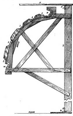
Fig. 2.-Mold for Running the Profile of the Ceiling.
