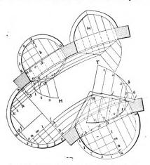
Fig. 9.-Welsh Groining on a Circular Plan,
