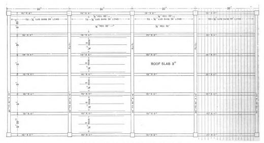
Framing Plan, Showing Reinforcement for the Roof.
