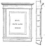
Elevation and Section of Medicine Cabinet in Bathroom.—Scale, 1/4 In. to the Foot.
