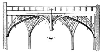
Fig. 20.—Sectional Elevation Indicating the Method of Construction.
