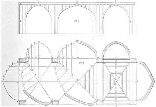
Fig. 5 .- A Groined Vault with Side Arches the Same Hight as Body Range but of Different Widths.
