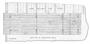
Partial Elevation of Wall Showing Method of Construction.
