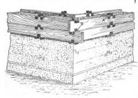
Fig. 2.—Manner of Using the Holders at the Corner of a Concrete Wall.
