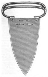
Novelties. — Iowa Concrete Cutter and Curbing Edger.—Fig. 4.—The Concrete Cutter.
