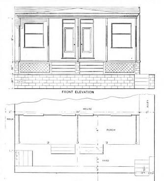
Improving the Appearance of a House Front.—Plan and Elevation of Porch.—Scale, 1/8 In. to the Foot.
