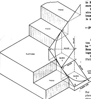
Fig. 76.—Isometric View of a Few Steps Within and Adjoining the Cylinder; the Sections Cut Through the Two Square Blocks; the Center Line of Wreath Lying on the Inclined Plane of Sections, Illustrating the Adaptability of the Operations to the Construction of Wreathed Handrails.
