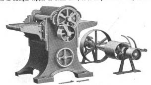
Fig. 7 .- New Wood Planer with Countershaft.
