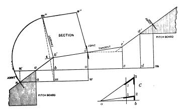
Fig. 78.—Elevation of Steps and Pitch of Tangents.
