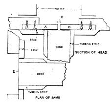
Details Showing Construction of Sliding Doors .- Submitted by "G. H. G."-Scale, 3 In. to the Foot.
