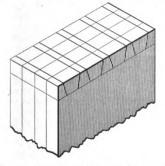
Fig. 39.—Showing Method Where Several Pieces of Same Size Are to Be Cut.
