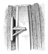
Fig. 4.—Running Stile by the Half Mold Method.
