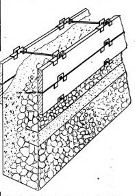
Fig. 3.—Holders in Use on a Straight Wall with Cobblestone Facing.
