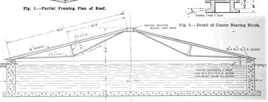
Fig. 2.—Sectional Elevation of Reservoir and Roof, Showing Truss Arrangement,
