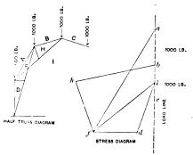
Stress Diagram and One-half of Truss Diagram.
