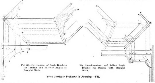
of the bracket, and the dotted lines u r, v s and w t show the manner of finding the bevel of the face. In the same figure is shown the manner of finding the bracket for an obtuse exterior angle. Let D I K be the exterior angle, bisect it by the line I G, which will represent the seat of the center of the bracket. The lines I H, m 1", n 2", o 3", o 4", o 5" are drawn perpendicular to I G, and their lengths are found as in the former case.
