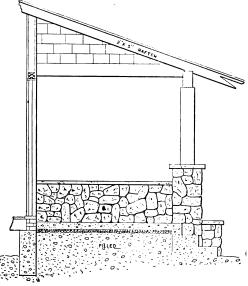
Section Through Front Porch.—Scale, 1/4 In. to the Foot.
