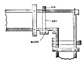
Fig. 5.-Manner of Constructing Corners.
