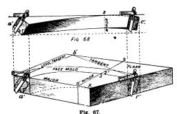
Fig. 67.—View of the Plank from Which the Wreath Is Cut Square to Its Surface and the Bevels Applied at Each End. Showing How the Wreath Is Twisted.
