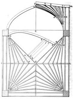
Fig. 17.—Another Example of Fan Tracery with Two Ribs Prolonged so as to Meet at the Ridge.
