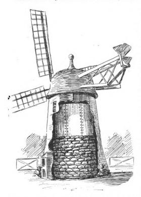
Fig. 3.—Broken View Showing Interior Storage Tank Placed on Stone Foundation.
