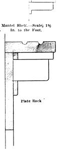
Details of Inside Finish and of Plate Rack .-Scale, 3 In. to the Foot.
