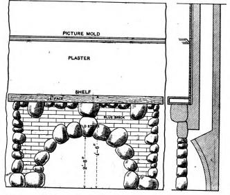
Elevation and Section of Fireplace in Living Room.—Scale, % In. to the Foot.
