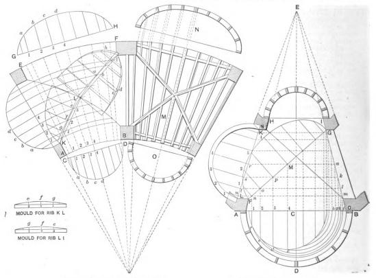
Fig. 13.—Groining on a Circular Plan.
