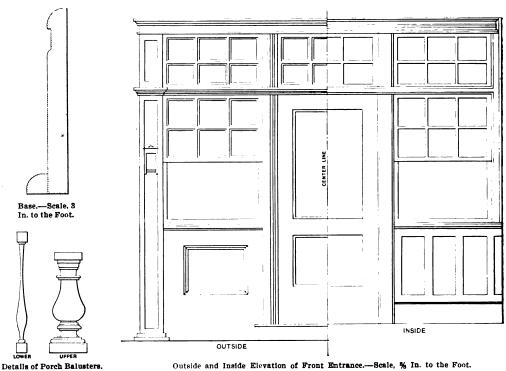
Outside and Inside Elevation of Front Entrance.—Scale, % In. to the Foot.
