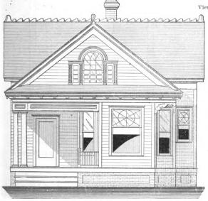
Front Elevation .- Scale, 1/8 In. to the Foot.
