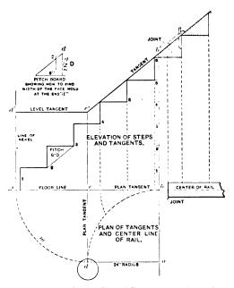
Fig. 2. Diagrams Showing Plan of Tangents with Center Line of Wreath; Also Elevation of Tangents and Steps.
