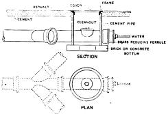
Details of Clean-Out at Rear Manhole Shown on Plan.—Scale, 1/2 In. to the Foot.
