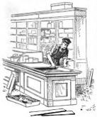
arrange them on the trestles in their proper order. If the material is quartered oak or other figured wood endeavor to place the pieces so that the figure will show to the best advantage and assist in concealing the joint. The board may be a few shades lighter on one edge than on the other. With a light and a dark edge together, no matter how good the joint it is always noticeable, while with the two light or the two dark edges together it may be made almost imperceptible.
