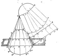
An Opening in a Straight Wall with Splayed Jambs and Circular Soffit Following Level at the Crown
