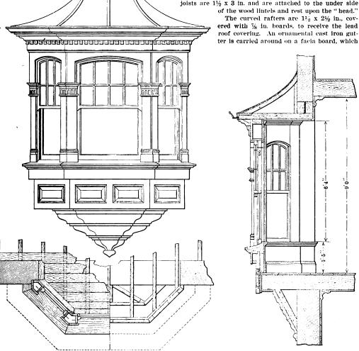
Figs. 1 and 2.-Elevation and Framing Plan.
