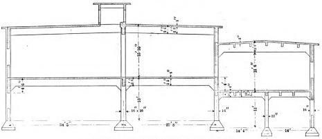
Cross Section Through Main Building and Lath Mill.
