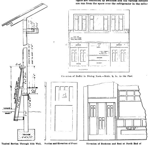
A Bungalow of Cement Plaster and Shingled Extertor .- Miscellaneous Constructive Details.
