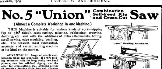
bination wood and iron table, 20 x 30°; rold-ing extension rolls for long work; two hand powers, one for self-feed ripping, and the other for cross-cutting, etc., arranged at rear of machine, leaving table free and allowing operator a natural, upright and easy position;
