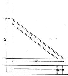
Fig. 2.—Plan and Elevation of Post Bracing.
