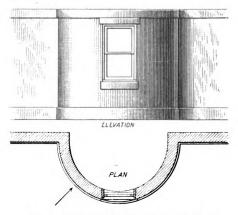
Fig. 4.—Method of Shading a Convex Surface.
