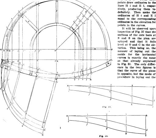
Fig. 34.-Sash for a Circular Wall with Cote Bars and Radial Bars with Circular Head Rail.
