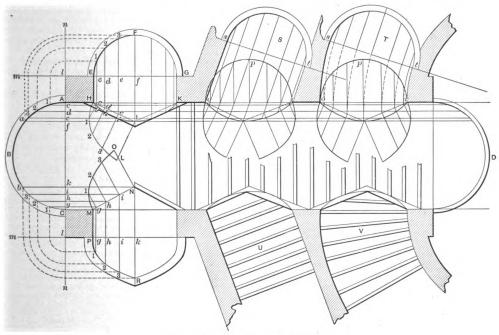
Fig. 7.-Four Examples of Welsh Groining.
