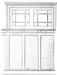
Detail Showing Plate Rack and China Closet in Dining Room.— Scale, % In. to the Foot.
