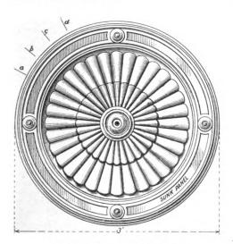
Fig. 1.—Simple Design for Centerpiece.
