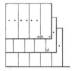
Fig. 4.—Corner of a Roof Showing How Shingles Are Laid.
