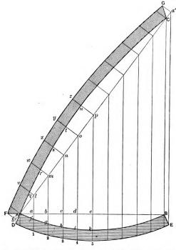
Fig. 33.—Method of Laying Out Face Mold for Diagonal Bar for
