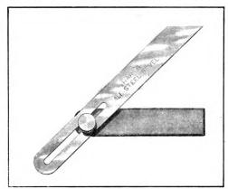
Fig. 6 .- Combination All Steel Bevel Try Square and Miter.
