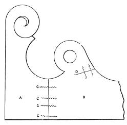
Fig. 10.-Showing Application of Corrugated Fasteners.
