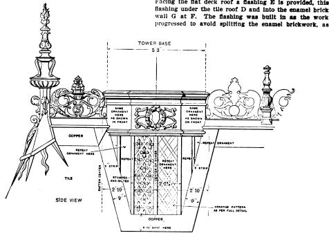
Fig 1.—Side Elevation of Cresting and Finials.
