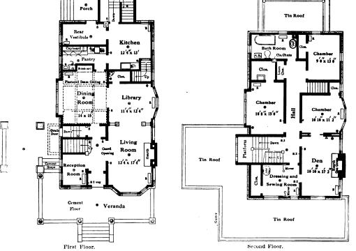
A House of Granite Face Brick-Tile Veneer .- Floor Plans .- Scale, 1-16 In. to the Foot.
