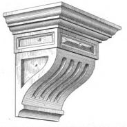
Fig. 1 .- Perspective View of Completed Plaster Truss.
