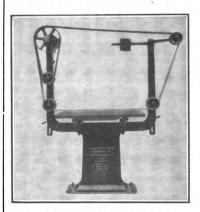
Fig. 5.—Universal and Flat Surface Sanding Machine.
