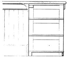
Fig. 35.—A Simple Design for Plain Work—Elevation and Section of a Counter that Can Be Bullt of Ordinary Stock.
