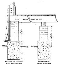
Details of Foundation.—Scale, 1/2 In. to the Foot.
