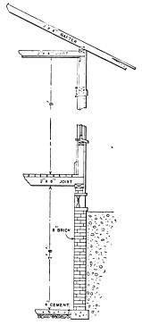
Section Through Rear Wall .- Scale, 1/4 In. to the Foot.
