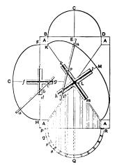
Fig. 2.—Diagrams Illustrating the Elliptograph or Trammel.
