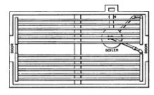
Fig. 3.-Graund Plan, Showing Piping.
