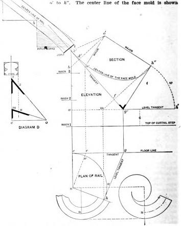
shown, it is located at the hight of 6 in. above the top of the curtail at Curve Greater Than a Quadrant, the Curve Being a Part of a Scroll.
