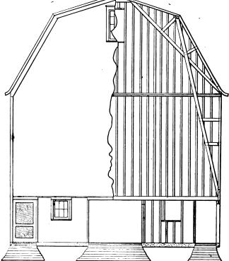
End Elevation, Showing Portion of Framing.—Scale, 3-32 In. to the Foot.
