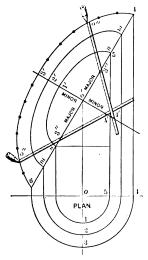
Fig. 48.—Showing How to Use the Straight-Edge to Draw Elliptical Curves,
