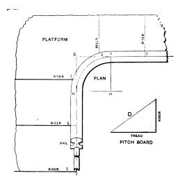
Fig. 43.—Pian of Stairway Having a Quarter Turn Cylinder Between Two Flights.
