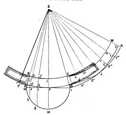
Fig. 27.—An Opening in a Circular Wall with Circular Soffit and Jambs Radiating to the Center from Which the Circular Wall Is Struck.
