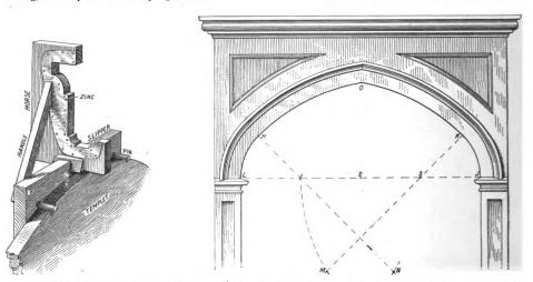
Fig. 7 .- View of Mold Showing Position of Pins on Template and Slipper Horsed to the Mold.
