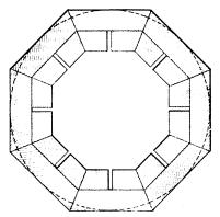
Remedying Trouble with Interior Hardwood Columns.— Cross Section Showing Saw Kerfs Somewhat Enlarged.
