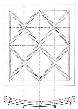
Fig. 32.—Sash on a Circular Plan with Diamond or Lozenge Shaped Panes.
