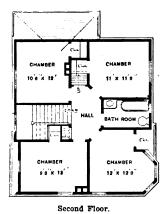
Design for a Low Cost Dwelling .- Floor Plans .- Scale, 1-16 In. to the Foot.
