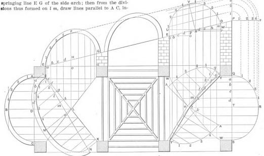
Fig. 6.—A Groined Vault with Imposts on an Incline.
