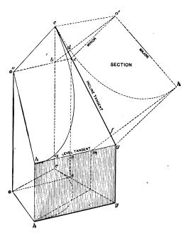
Fig. 64.—A View of Fig. 60 Folded in a Solid Block, Showing Graphically the Method of Developing a Section Cut Oblique to One Side and Its Application to Handrailing.
