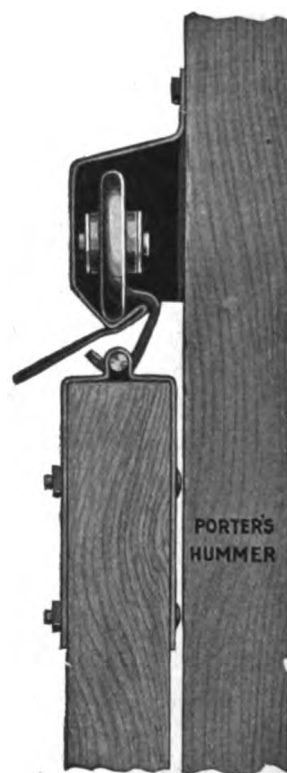
Fig. 4—Vertical Cross-Section Showing Hanger in the Groove
