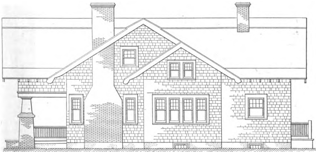
Side (Right) Elevation Showing Outside Chimney—Scale 3/32 In. to the Foot
