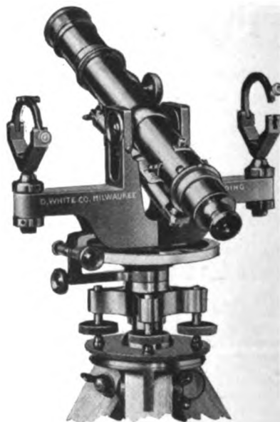
FIG. 6—The Instrument When Used as a Transit
