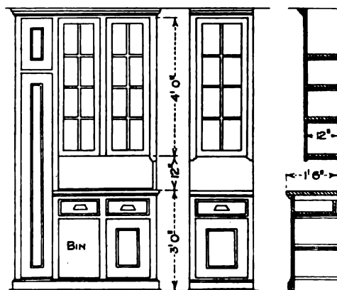
Section and Elevations of Kitchen Cupboards—Scale \frac{1}{4} In. to the Foot
