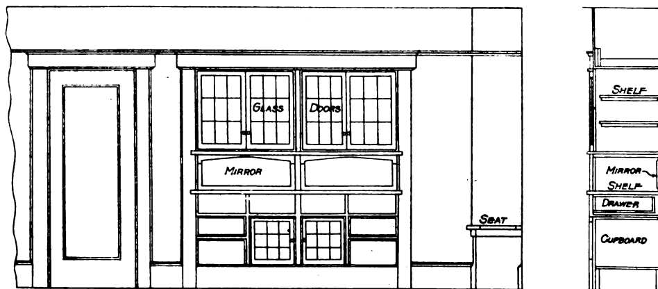
Elevation of Wall in Dining Room Showing Built-in Buffet with Vertical Section—Scale \frac{1}{4} In. to the Foot
