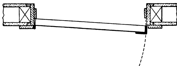
Fig. 1—Method of Finding Bevel for Edge of Door
