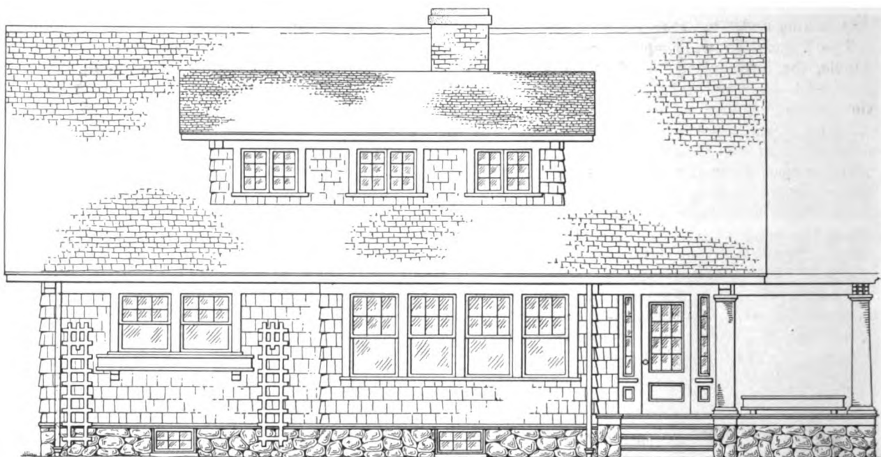
Front Elevation Showing Some of the External Features of Architectural Treatment—Scale \frac{3}{32} In. to the Foot
